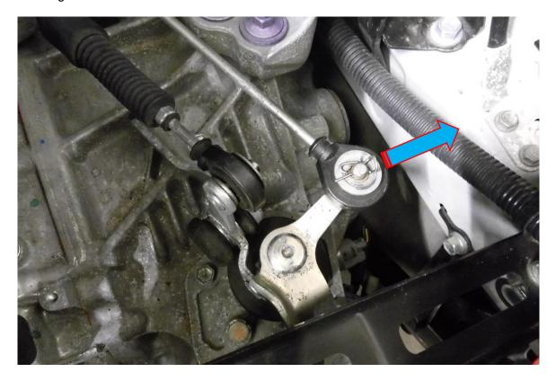
6. Insert the shifter pin and M8 nut into the FMSS5 body as shown in the picture below, adjust the shift pin back and forth until the desired position is found. Use a 16mm spanner to secure it place.
