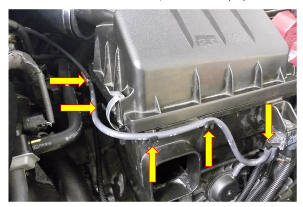
4. Push the retaining tab inwards on the loom to the airbox pump and unplug from the pump, then unclip the loom which is attached to the airbox. The airbox will now pull out of the engine bay.
