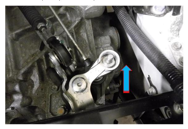
9. Place the machined locking nut from the FMSS5 kit through the gear box linkage pin and screw it to the FMSS5 body hand tight, then nip it up using a 16mm spanner or socket and ratchet.
