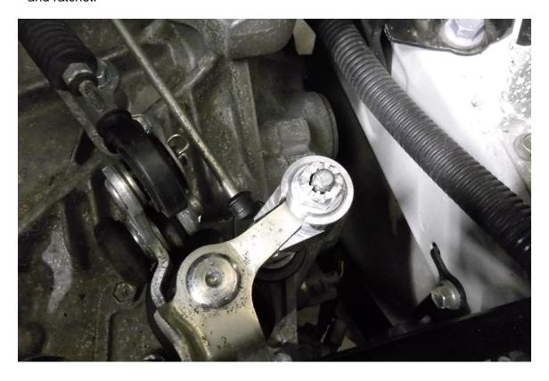
10. To lock the nut into position, use the supplied split pin. Make sure the split pin passes through two of the groves in the FMSS5 nut and through the hole of the gearbox linkage pin. You may have to adjust the nut, so it lines up.
