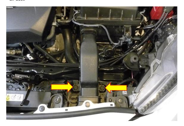
2. Using a 7mm or 10 mm socket and ratchet loosen both hose clamps of the inlet hose which will allow you to remove the hose from the airbox. Press in the retaining tab on the MAF loom and unplug it from the MAF.
