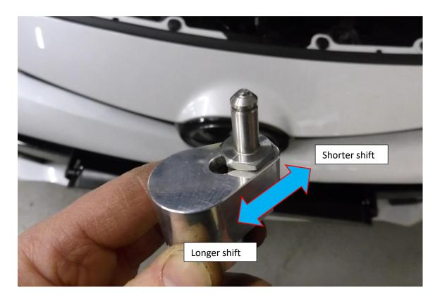
7. Fit the FMSS5 to the gear shifter rod as shown in the picture below. Secure it to the gear shifter rod with the supplied side retaining clip.
