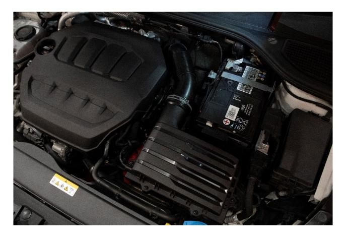
2. Using a hose clamp removal tool, slide back the hose clamp as pictured below and disconnect the inlet hose from the airbox.
