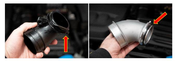
8. Fit the Forge Motorsport turbo elbow into position and rotate anti clockwise.
