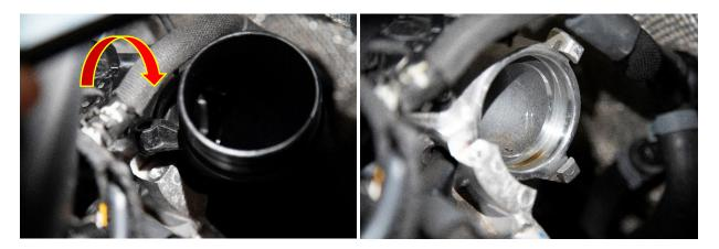
7. Remove the o-ring from the OEM elbow and fit onto the Forge Motorsport item as pictured below.
