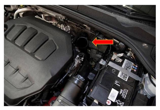
5. Using a T30 torx drive and suitable rachet remove the fastener that holds the turbo elbow in position.
