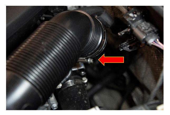
4. Locate the turbo elbow, towards the front of the elbow is a T30 torx fastener.
