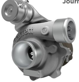
Garrett Boost | Club Line turbochargers are engineered for small engine displacements including powersports, personal watercraft, and automobiles. These turbochargers feature internally wastegated turbine housings and journal bearing rotating groups. Forged, fully-machined compressor wheels can support from 200 up to 350 horsepower for engine displacements ranging from 0.4L up to 2.5L
