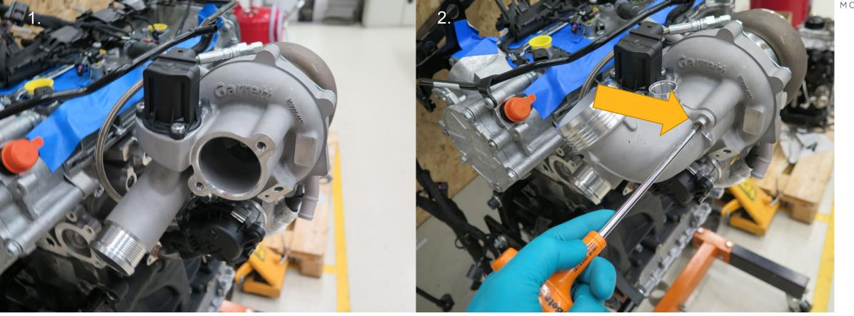
1. Use provided inlet adapter, gasket, and 2 M8 x 20 supplied bolts to attach to the compressor inlet
