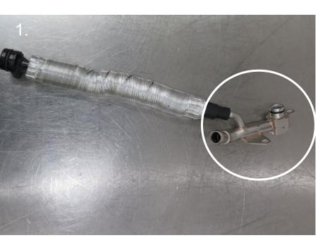
1. Remove turbo connecting pipe
