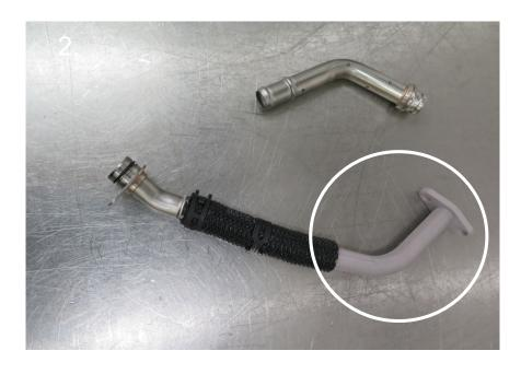
2. Replace with provided oil drain tube
