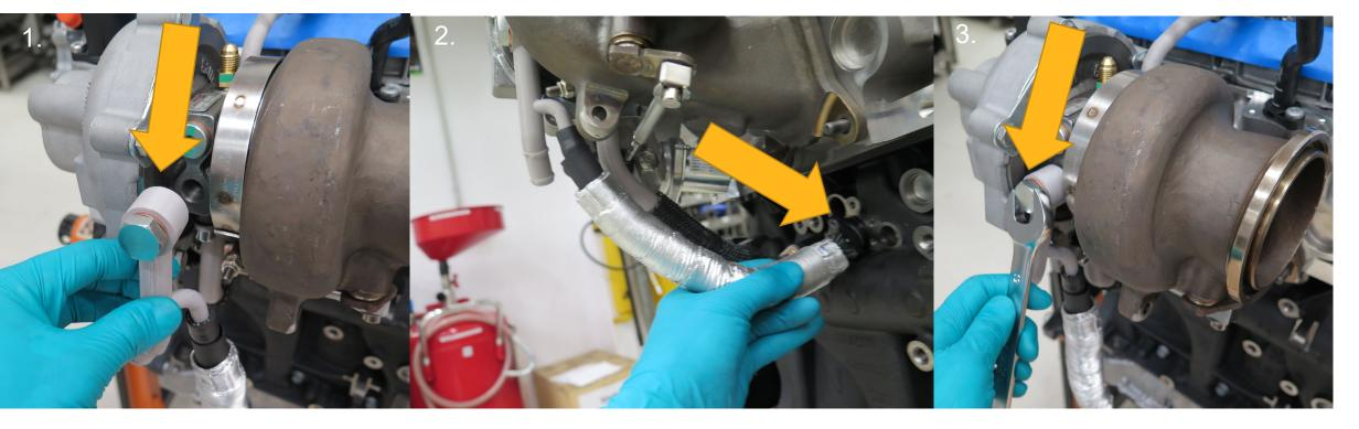
1. Attach water inlet tube to the turbo with provided banjo bolt and copper washers. Engage threads with fingers.
