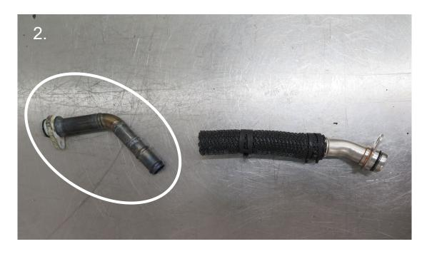
2. Replace with provided pipe and check hose clamp to ensure a tight connection
