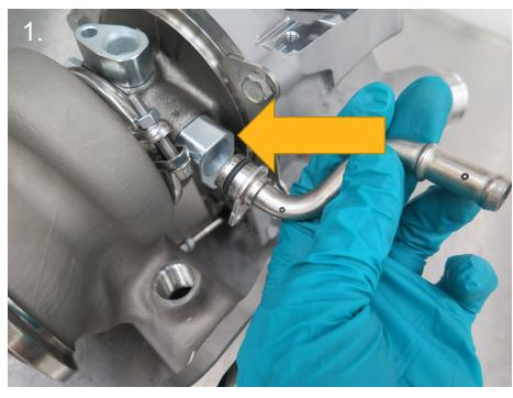
1. Lubricate water outlet pipe O-ring and press into the water outlet adapter
