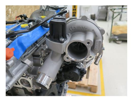
1. Use provided inlet adapter, gasket, and 2 M8 x 20 supplied bolts to attach the compressor inlet
