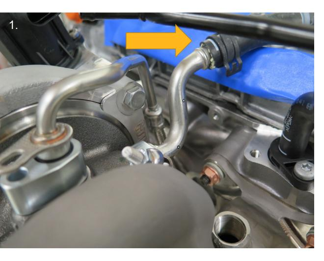
1. Connect water outlet to OE engine hose and tighten clamp
