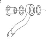
2. Attach lower hose to the engine using the OEM bolt. Tighten to OE specifications.
