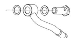
3. Turn banjo bolt with fingers to engage threads into the turbo housing. Torque to 20Nm / 14.75ft-lb
