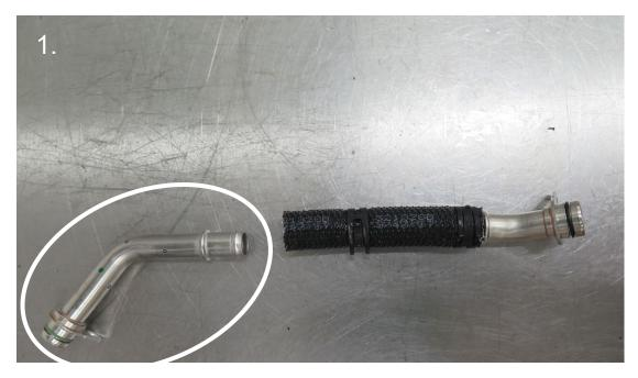
1. Remove OEM connecting pipe
