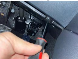
Fold the cover down and find the OBD port as well as the hole right next to it. This is where we route the cable through.
