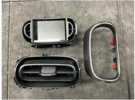
The cover fits the CANchecked unit exactly the same way. Slide the cover over the display unit and make the tabs click into their place.
