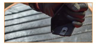
7. Install the small bracket to the studs on the firewall. (2x 10mm nuts)
