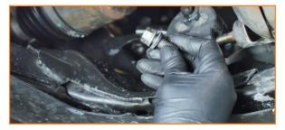
10. Angle the larger bracket in your kit up into the engine bay. Install the larger bracket to the steering rack using the same bolt from the previous step. Do not fully tighten the bolt yet. You will return to this later. (1x 14mm bolt)
