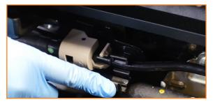
Remove two bolts behind the fuel line. (2x 10mm bolts)
