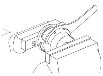
Reinstall fittings to the cap of the Raceport using fresh Loctite 567 thread sealant.
