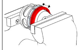
Inspect for Damage before inserting piston assembly into Raceport Body. Ensure Diaphragm bead is seated correctly in the groove on the body.
