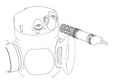
Tighten the new solenoid into the EM series BOV ensuring the wrench is on the metallic portion of the solenoid.
