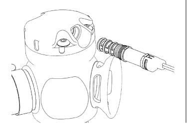
Tighten the new solenoid into the EM series BOV ensuring the wrench is on the metallic portion of the solenoid.
