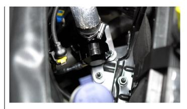
**Congratulations**, your EM Series BOV is installed and ready for use. Double check all electrical connections and fasteners.
