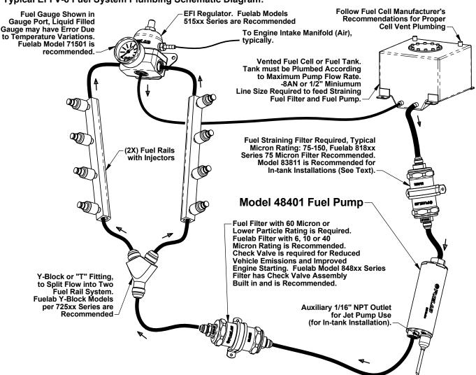
Special Note: Use in carbureted systems require a bypass return or relief valve.
