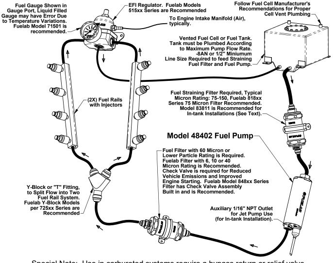
Special Note: Use in carbureted systems require a bypass return or relief valve. Do not "Dead Head" Fuel Pump.
