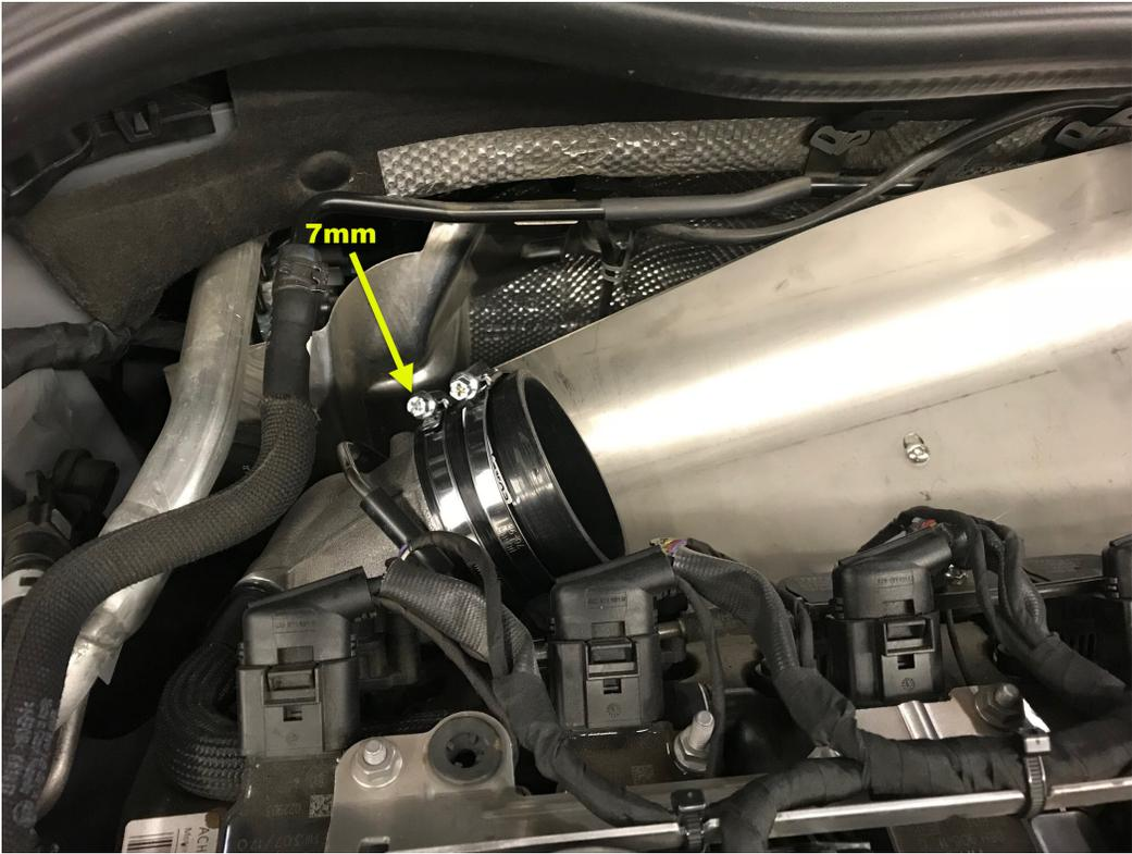
**Step 16** – Insert intake tube through the hole in the carbon fiber airbox frame.
