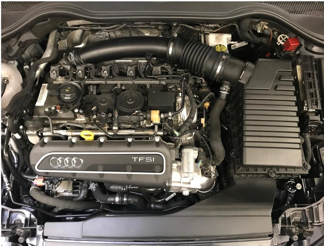
**Step 3** – Using a pair of pliers, loosen the spring clamp on the bypass hose and disconnect hose from OE intake. (For 2019+ vehicles, use a 5mm Allen to disconnect the bypass hose from the OE intake tube by removing the two Allen bolts.)
