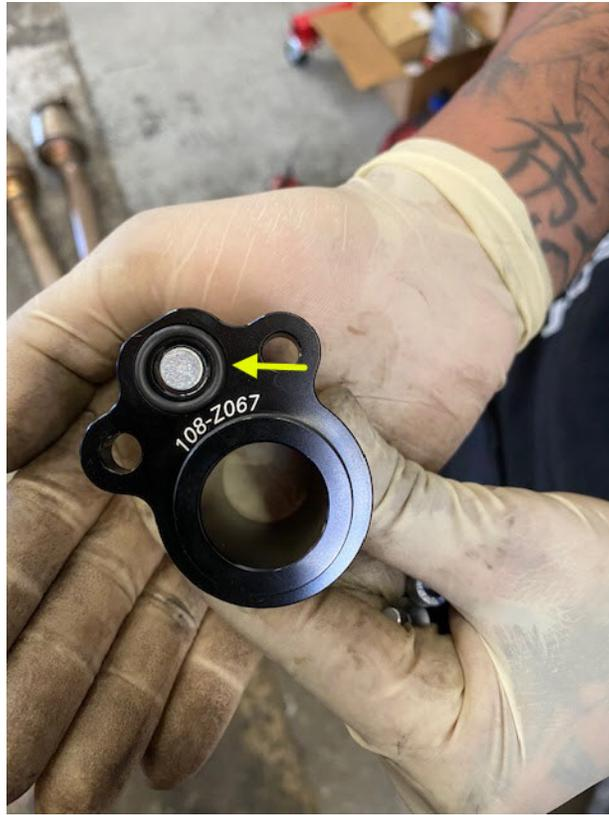
**Step 17 (2019+ vehicles)** - Re-using the OE socket head screws, install the supplied adapter, being careful not to lose the small o-ring.
