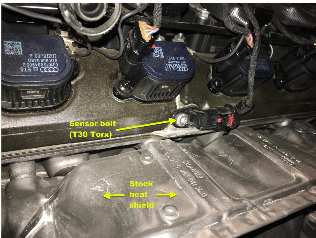
**Step 13** - Using a 4mm Allen wrench and the supplied M6 button head cap screws, assemble heat shield.
