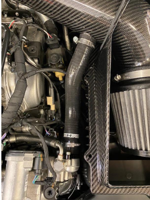
**Step 23** – Tighten hose clamp at the silicone coupler (see image in Step 19).
