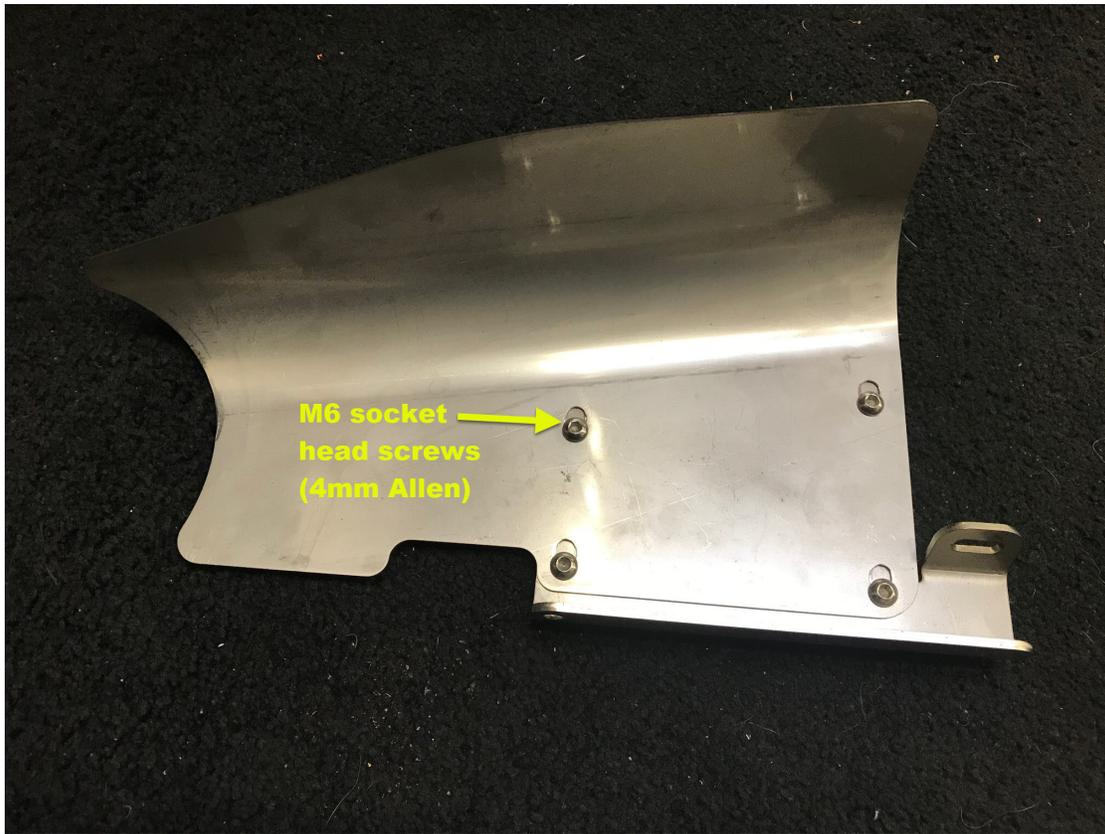
**Step14** - Install the heat shield by attaching to the stock intake tube mounting bracket (Step 6), and the head sensor (Step 12). Shield location can be adjusted by loosening the M6 button head cap screws. Make sure wiring along the firewall does not contact the edge of shield.
