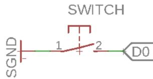
digital inputs D0-D8 are provided with a pull-up.
