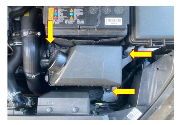
6. Using a 10mm socket and ratchet remove the M6 fastener from the air duct shown in the picture below.
