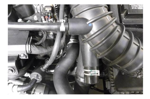
2. Using a 10mm socket and ratchet loosen the hose clamp attaching the inlet hose to the airbox, once loose detach it from the airbox.
