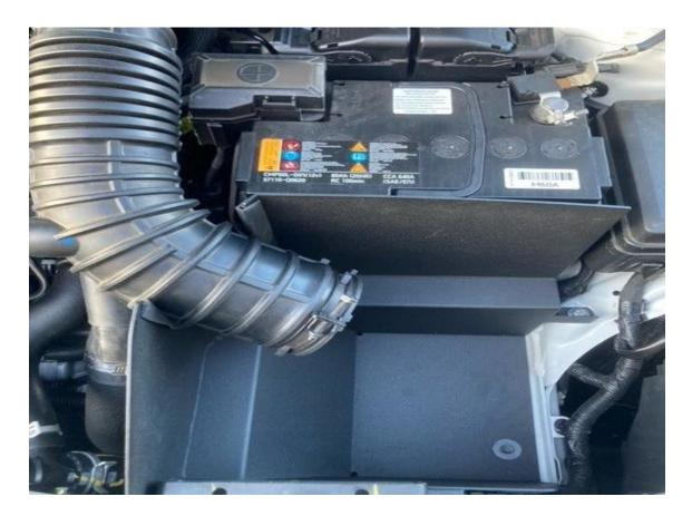
**11**. Attach the smaller 76mm end of the angled hose joiner from the kit to the intake hose, but do not tighten it in place just yet.
