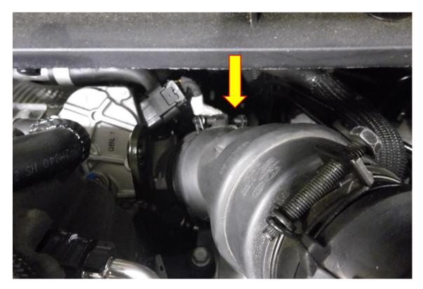
4. Using a flat bladed screwdriver prise the X2 plastic retaining clips open and remove them from the air duct to the airbox.
