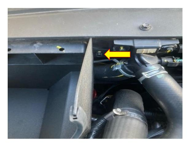
9. Pinch the tabs inwards to release the retaining clips on the actuator and lambda wiring looms to remove the bracket.
