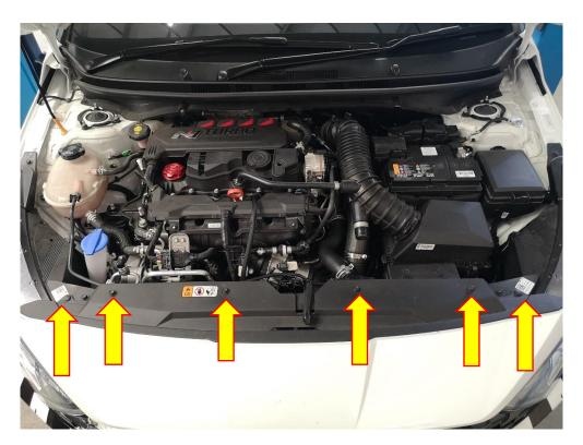
3. Using a trim tool or flat blade screwdriver remove the three clips on the inside of both wheel arches. Using an 8mm socket and suitable drive or Phillips screwdriver remove the fastener at the top.
