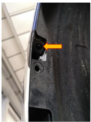
4. Using a trim removal tool or flat blade screwdriver remove the 11 plastic fasteners from the under tray.
