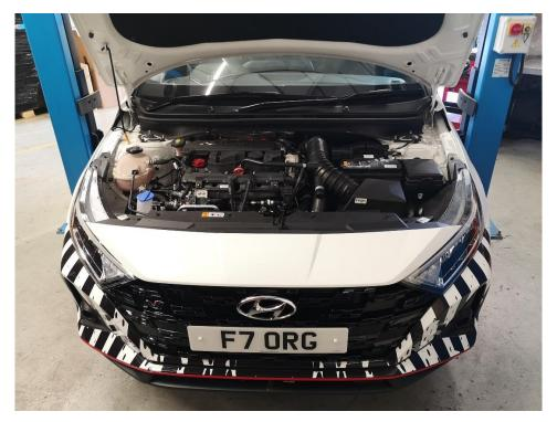
2. Using a trim removal tool or flat blade screwdriver lift the centre of the two plastic fasteners each side of the slam panel. Using a 10mm socket and appropriate drive remove the 4 bolts along the middle of the slam panel.
