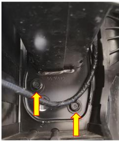
9. Using either a 10mm socket and suitable drive or Pozi drive screwdriver undo the 4 bolts that hold the plastic trim around the stock intercooler. You can then pull this towards you to remove from the vehicle. Due to the increase in size of the Forge Motorsport intercooler this trim will not be re-fitted to the vehicle.
