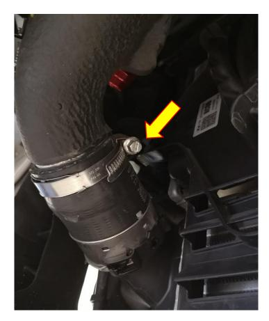
**11**. Using an 8mm socket and suitable drive undo the hose clamps to hose A at both ends and remove it from the vehicle as shown below.
