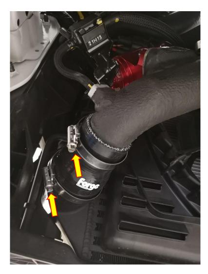
17. Using a 7mm socket and suitable drive tighten hose #2069 with a 40-60mm and 50-70mm hose clamp between the boost pipe and intercooler as shown below. You may find silicone spray is helpful when installing.
