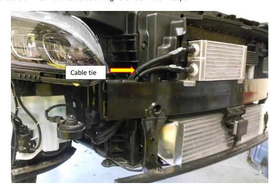
23. Add 500ml of the appropriate grade engine oil to your vehicle to compensate for your new Forge oil cooler. Now start the engine, get it to full running temperature and check for oil leaks, if you do find any leaks; wait for it to cool down and tighten fittings accordingly.
