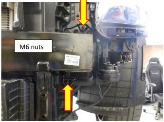
9. With the crash bar removed fit the supplied rubber edge trim to the offside of the radiator cowling. Using a drill with a 6mm drill bit make a hole on the radiator pack fin as shown in the picture below. The hole will be used for securing the oil cooler lines at a later stage.
