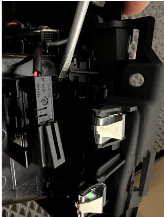
On the underside there is also a latching nose. If this is also loosened, the ventilation grille can be removed from the shaft.
