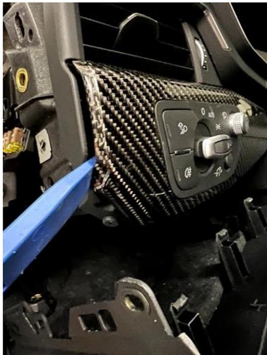
After the aperture is released, it can be packed left and right and carefully pulled out of the shaft. Please remove the rear plug to remove the bezel.
