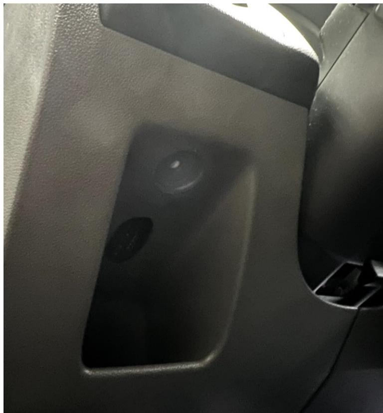
Now a hole must be drilled into the fairing with a drill. Here an 18mm hole or two, with the file to a slotted hole worked out 10mm holes next to each other is sufficient. The hole must be large enough to fit through the eight- and ten-pin Molex connector from the OBD cable.
