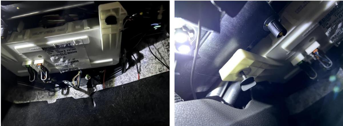
In the connection, the fuse box can be folded downwards.
