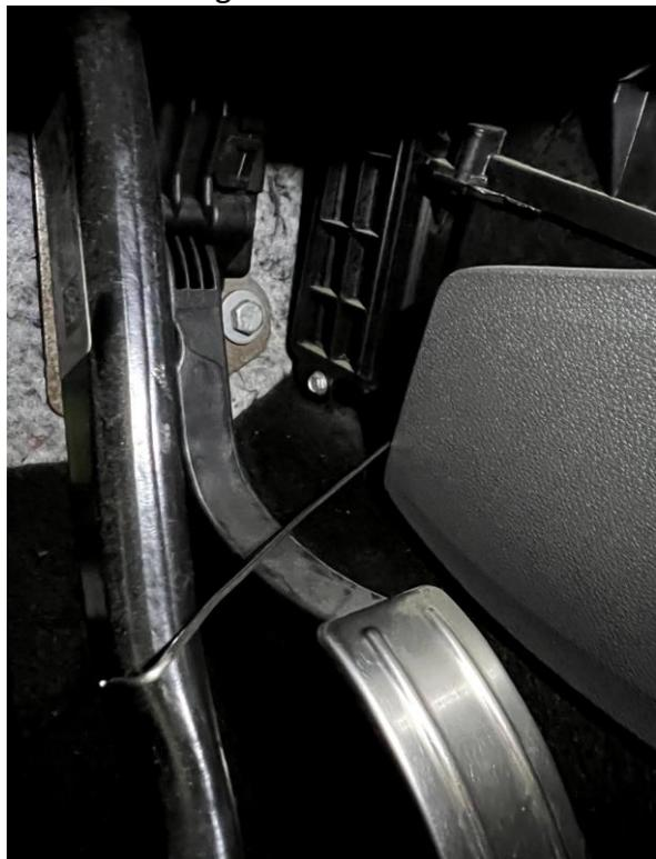
The cable coming from the fuse holder is now also crimped with the red cable on the OBD connector. This line later supplies your data display with ignition plus. When laying the cable, care must be taken to ensure that the cable cannot be jammed.
