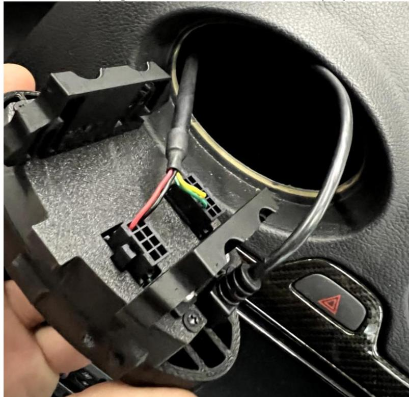
Now the display can be carefully inserted into the position in the ventilation, and then the bezel can be clipped in.
