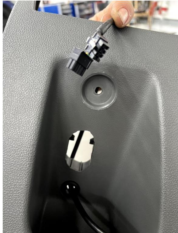
Next, the fairing in the passenger footwell must be removed. This is also secured with a screw.
