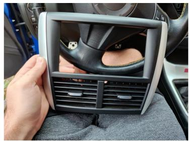
After removing, slightly lever up the 4 marked holders on the back to remove the ventilation duct.
