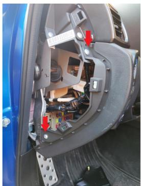
Now remove the fairing under the steering wheel, which is now only attached by clips, pull the fairing off carefully. Before you take it off completely, disconnect the connectors.
