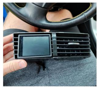
Now you can, before you reassemble everything in reverse order, briefly switch on the ignition and check the display for function. If this is given, you can complete the vehicle and you are done.
