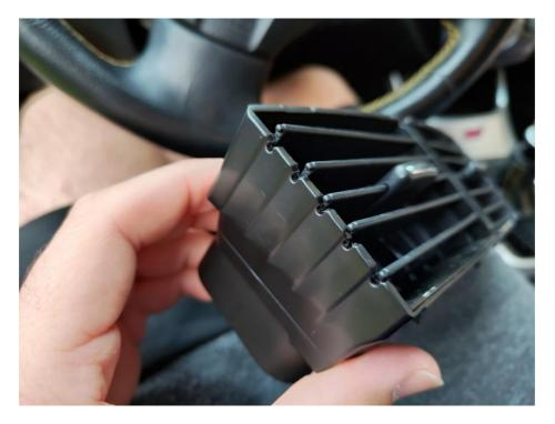
Then it's time for the rear lamellas. To do this, place your fingernail between the two plastic edges and press against the lamellas from behind.
