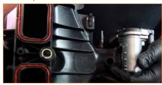
CAPTION: The PCV port on the back of the intake manifold is not visible while the intake is installed on the vehicle.
