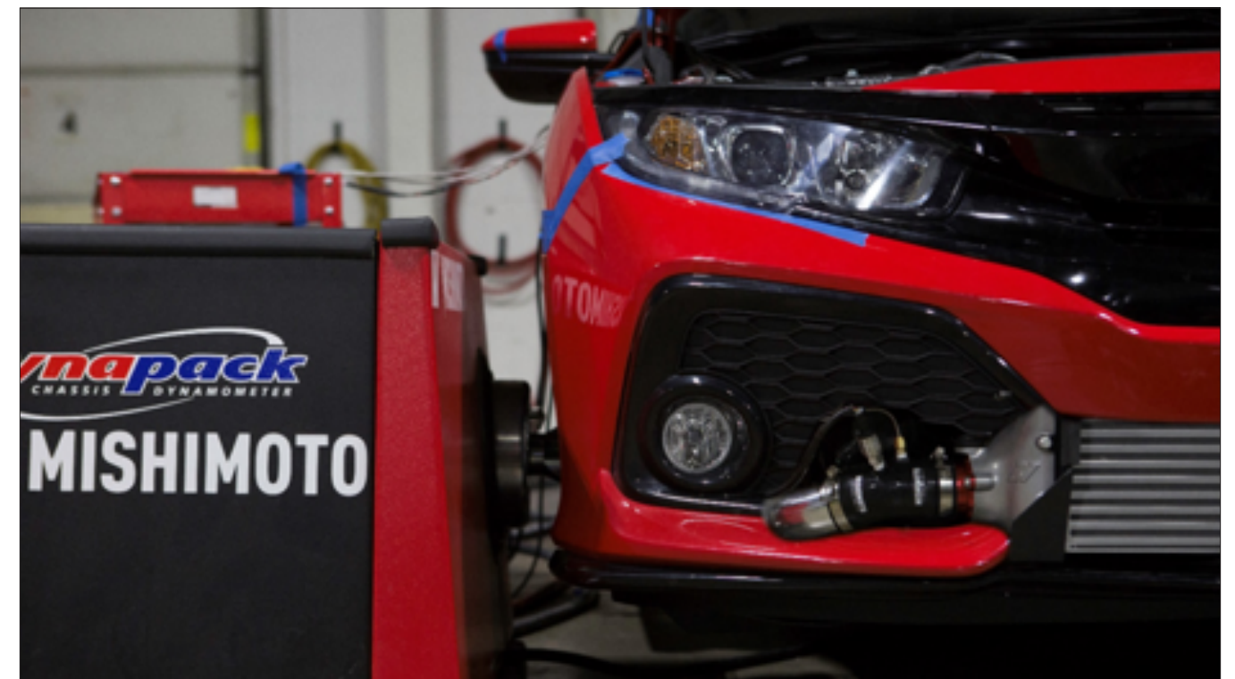
FIGURE 6: Pressure and temperature sensors installed in hot-side intercooler pipe.
