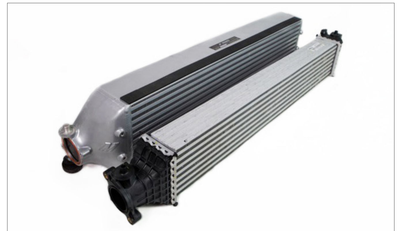
FIGURE 3: Comparison of the stock intercooler to the Mishimoto intercooler.
