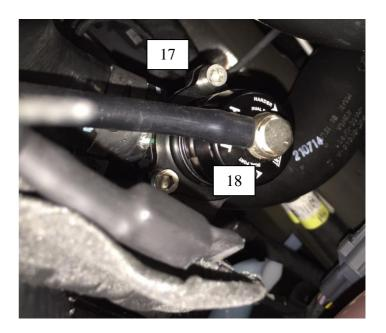
19. Install provided electronic plug onto OEM solenoid plug as shown. Secure with cable ties.
