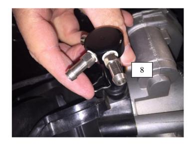
9. Once installed, the boost reference adapter should look as shown. Vacuum hoses can now be connected.
