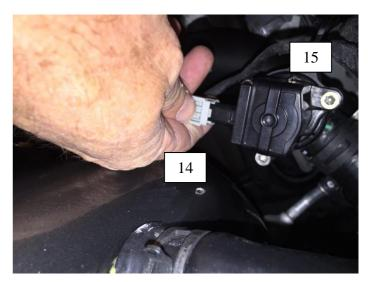
16. Install your new Turbosmart BOV. Align the mounting holes with the flange. As can be seen in the image, the plumb back port of the blow off valve should be facing the plumb back pipe. Holes are not evenly spaced. The BOV will only be installed in one way. Do not force the BOV in, damage will result.
