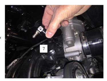
8. Install the retaining clip provided to secure the boost reference adapter in position
