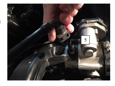
6. Cut and remove the OEM line as shown.
