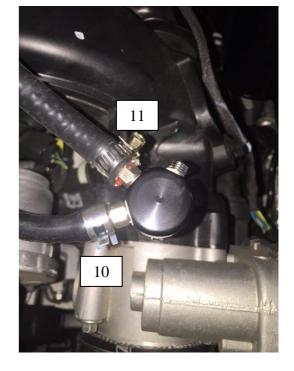
12. Install other end of ¼" re-inforced hose over barbed end of PCV check valve as shown. No clamp is needed.
