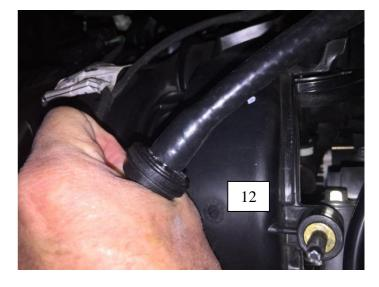
13. Once installed, the boost reference adapter and hose should look as shown.
