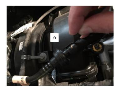
Slide the boost reference adapter onto the OEM port as shown. Twist adapter back and forth while pressing down as there will be some resistance due to the internal O-ring.
