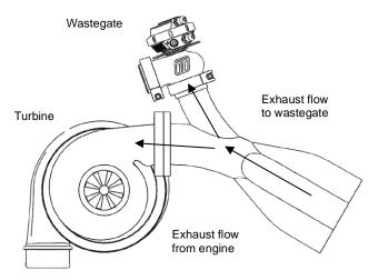
Figure 4 - Best flow - Symmetric mounting
