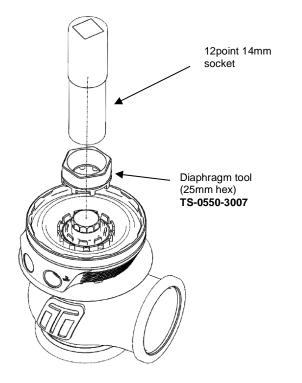
Clear any Loctite and debris from the thread in the diaphragm support, Note careful not to get chemicals onto the diaphragm as this may damage the diaphragm.
