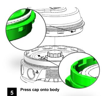
Using a press or vice, compress the cap onto the body ensuring the notches are remaining aligned, use spacers to ensure the wire from the sensor it not crimped or damaged Once the cap has seated home onto the bod, screw the collar down by hand in a clockwise direction. While still in the press or vice, Tighten the collar further with the collar tool until the collar will not turn.
