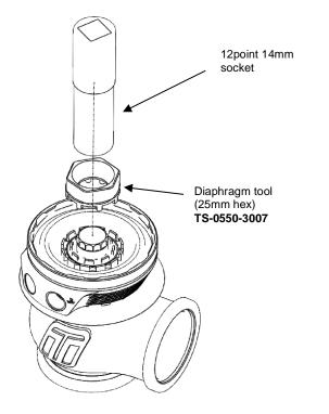
Remove the valve retaining cap and spring washer, Sit the wastegate on down so that the valve is elevated and supported. Using a small flat blade screwdriver to pry one edge of the split in the valve circlip out and up, work your way around the circlip until it is removed. Take note of the orientation of the diaphragm, lift the old diaphragm over the valve and discard. Use this opportunity to thoroughly clean the wastegate removing any dirt from the actuator, ensure the diaphragm over the valve.
