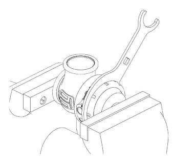
Reinstall fittings to the cap of the wastegate using fresh sealant.
