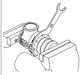
Reinstall fittings to the cap of the wastegate using fresh Loctite 567 thread sealant.
