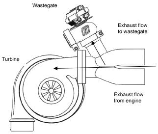
Figure 5 - Good Flow - Angle mounting
