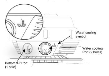
Fit water cooling port fittings Prior to mounting the wastegate, install 1/8" NPT fittings into the water ports, apply thread lubricant and screw in clockwise until finger tight, then tighten further 1-2 turns for seal. Choose feed and drain source for the water and connect to the wastegate. Turbosmart recommends -4SAE fittings and hose compatible with coolant.
