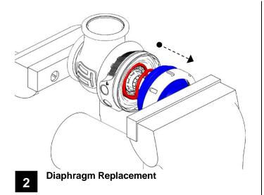
Use the supplied tool in the diaphragm replacement kit, engage the diaphragm aligning the splines and grooves. Use a 25mm spanner on the tool to prevent the diaphragm from spinning. Use a 12point 14mm socket through the centre of this tool onto the valve retaining cap. Undo the valve retaining cap by rotating in an anti-clockwise direction.
