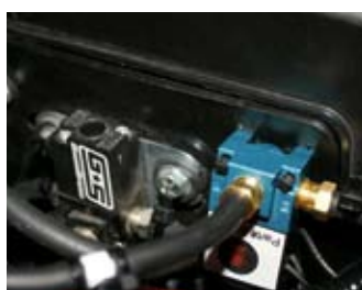
Mounting Example Mazda 3 (SI-Solenoid)
