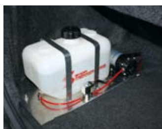
Mounting Example Nissan 370Z Driver's side trunk compartment
