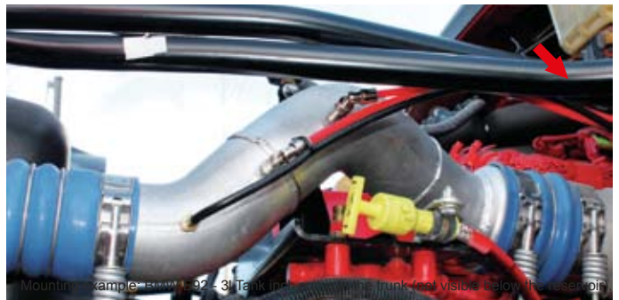
Mounting example 8.3l Cummins Diesel. Boost source adapter (left) and 2 installed nozzles.
