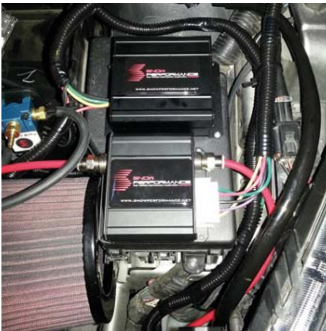
SafeInjection- and Stage 2 Controller in the engine compartment (Mazda 3 MPS)
