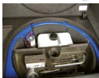
Mounting Example Audi A6 Spare Wheel Recess
