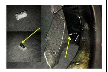
6. Behind the lamp, there will now be a metal stud visible. Using a 10mm hex head deep socket, remove the nut. (Repeat for each side of the vehicle, 2 in total.)
