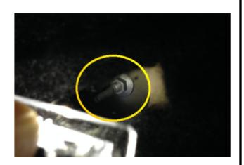
7. The rear bumper cover should now be completely loose. Before removal from the vehicle, be sure to carefully slide the plastic diffuser panel downward, releasing it from the 3 metal studs on the underside of the car.
