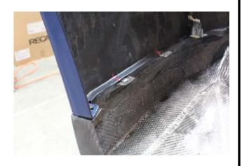
12. Once fitted, attach the provided speed nuts [U-Clips] to each of the tabs along the back edge of the diffuser (9 total) and use the included screws to pass through the OEM tabs and into the speed nuts.
