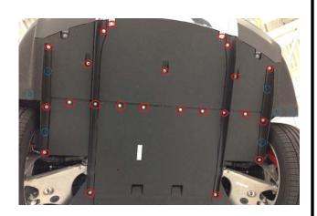
15. Remove the rear reflectors from the OEM rear under spoiler by pressing firmly on the backsides of each of the tabs. Install reflectors into U.P. Rear Under Spoiler using the OEM tabs.
