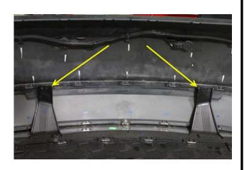
10. The rear under spoiler should now be loose. Carefully pull the rear under spoiler toward the visible end of the rear bumper cover, separating it from the bumper cover.
