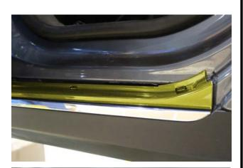
2. Next located the body-painted plastic finishing strip (highlighted in yellow). This strip is attached the OEM rocker molding using metal clips. Using a plastic panel tool, pry firmly away from the body of the car. Each of the metal clips should pop loose.
