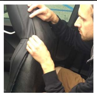
8. Press the trim strip firmly into the slot / seam around the seat back.
