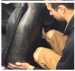
7. To replace the OEM leather trim attachment strip, begin around the top of the seat.
