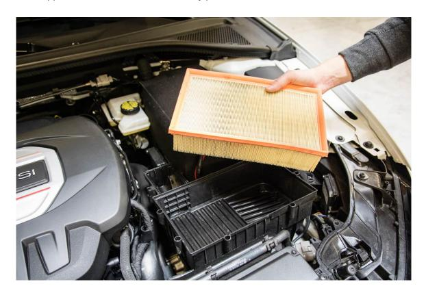
**Step 7** – Remove the air baffle from the factory lower air box. **Note:** This piece has tight tolerances within the air box, and will take some wiggling and coaxing to remove. This baffle will not be used when installing the 034Motorsport MQB P34 Intake System.
