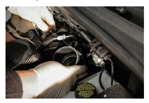
**Step 12** – Install 034Motorsport High-Flow Panel Air Filter into factory lower air box. **Note:** Be sure filter is seated and flush with the factory lower air box.
