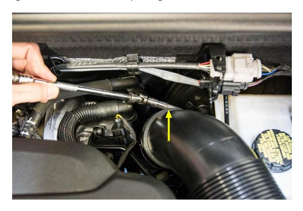
**Step 5** – The air box should now be completely free. Lift up and away to remove the upper air box and factory inlet tube from the engine bay.
