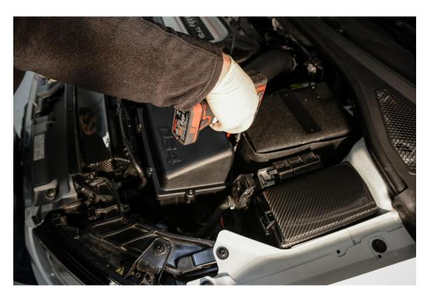
**Step 15** – Install the factory vent hose to the nipple fitting on the left side of the 034Motorsport MQB P34 Intake System.
