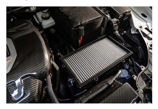
**Step 13** – Once the air filter is installed in the factory lower air box and silicone coupler are secured to the turbo inlet pipe, place unit on top of factory lower air box and align inlet tube with turbo inlet. After aligning the other side of the intake with the lower air box, tighten and secure the hose clamp holding the silicone coupler to turbo inlet and air box using a Flathead Screwdriver.
