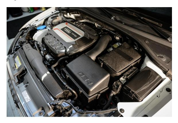
**Step 14** – Install 6 of the 8 factory Torx screws and washers to secure the 034Motorsport MQB P34 Intake System to the factory lower air box. Torque screws to 4 Nm with a T25 Torx.
