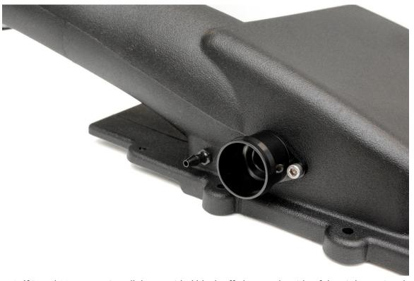
**Step 10** – For Golf R and S3 owners, install the provided block-off plate on the side of the air box using the supplied allen bolt. Torque bolt to 4 Nm using a 4mm Allen key.
