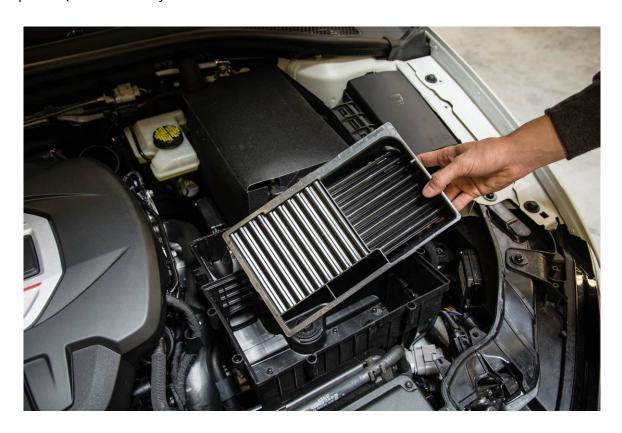
**Step 8** – The 034Motorsport MQB P34 Intake System includes a provision for the airbox-mounted secondary air injection fitted on Golf, GTI, and A3. For those with a Golf R or S3, a block-off plate is provided in the kit to eliminate the SAI provision.
