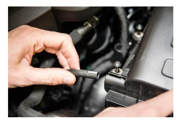
**Step 4** – Using a 7mm socket, loosen the hose clamp securing the inlet tube to the turbo.
