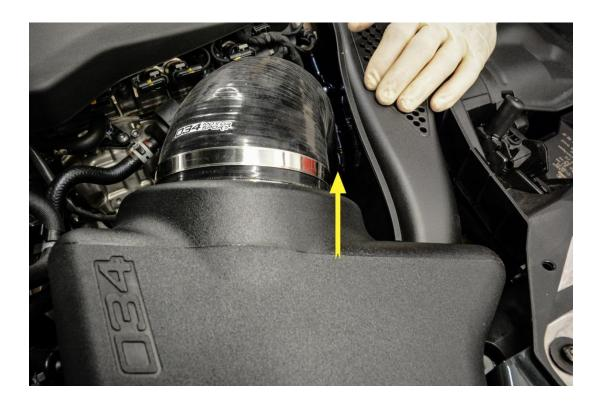
**Step 16 –** Using a 8mm Hose Clamp Driver or Socket, tighten the hose clamp securing the inlet hose to the air box.
