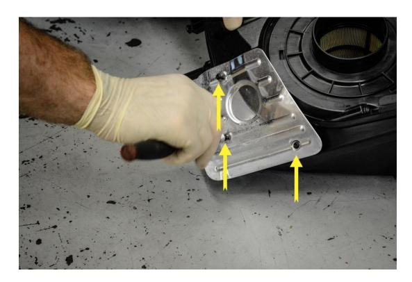
**Step 10** – Install the factory heat shield on the 034Motorsport P34 Cold Air Intake air box using 2 of the factory screws and a T20 Torx.
