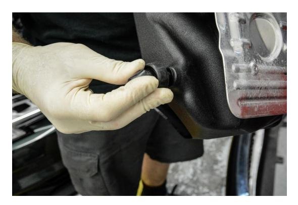
**Step 12** – Tip: Spray the rubber grommets with a lubricant to help them seat properly in the engine bay when installing the air box.
