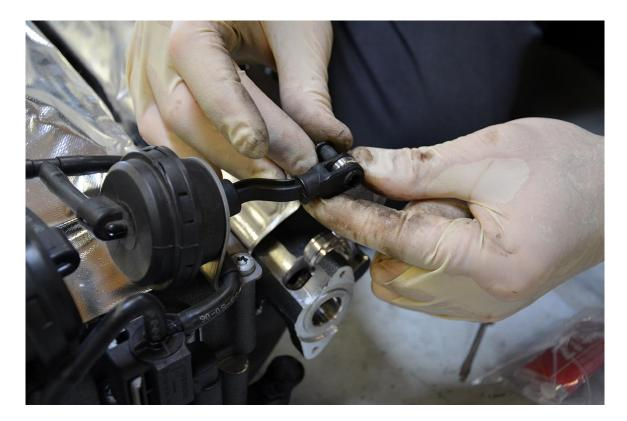
**Step 13** – A set of channel lock pliers may be used to ensure that the plastic pin is fully seated.
