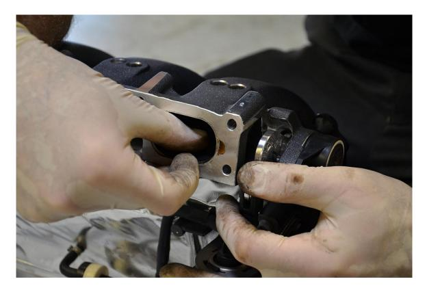
**Step 19** – Apply Loctite to the threads of the T20 Torx screws you removed from the intake manifold flaps/rods in <u>Step 3</u>, and use them to secure the flaps to the rod.
