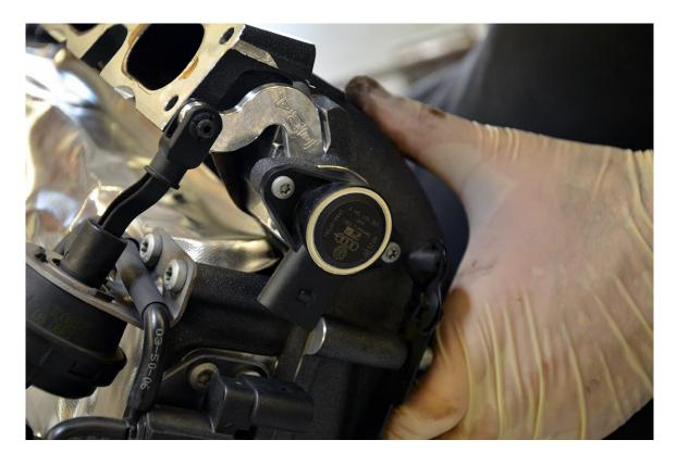
**Step 18** – With the intake manifold on its side, gently place the intake manifold flaps into the ports, aligning the holes on the flaps with the threaded holes in the intake manifold flap rod.
