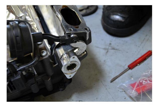
**Step 15** – Once the intake manifold flap rods are installed, check to make sure that they are centered. This is done via the small hole you removed the retaining plug from in <u>Step 5</u>.
