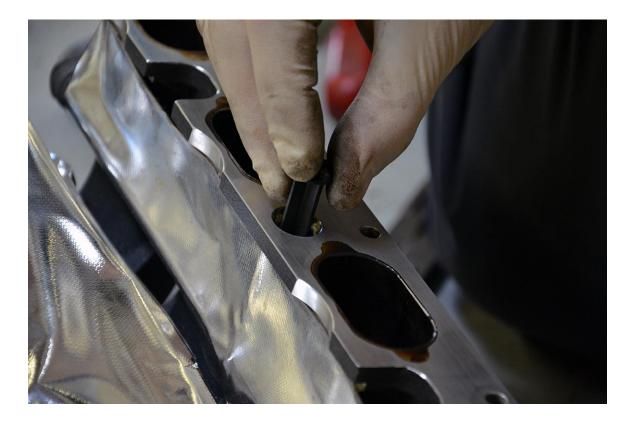
**Step 17** – Reinstall each of the intake manifold flap sensors to the intake manifold, and secure each using two T20 Torx screws. We recommend tilting the manifold on its side to reinstall the flaps in the following step.
