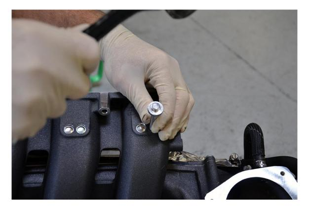
**Step 2** – Continue removing the intake manifold plugs until you've removed all 16 of them. Set the plugs aside for reinstallation later. Pat yourself on the back – you deserve it!
