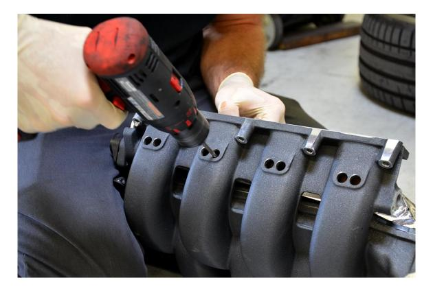
**Step 4** – Remove each of the intake manifold flaps through the intake manifold ports. There are 8 in total. **Do not lose any of them!** You're already keeping track of 40 things you don't want to lose, so give yourself another pat on the back. Excellent work!
