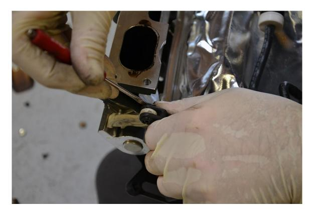
Step 8 – Once the plastic pins are removed, set them aside for reinstallation. Do not lose either of them!
