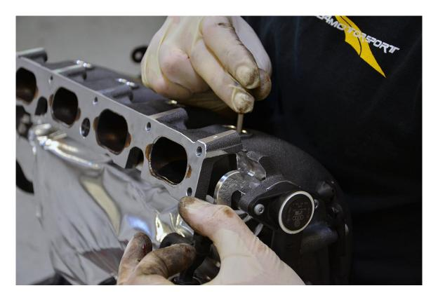
**Step 20** – Apply Loctite to the intake manifold plugs you removed in <u>Step 1</u>, and gently tap them in using the shorter (small) end of the supplied Intake Manifold Plug Installation Tool. **Do not use the longer end for this!** The stop on the short side is designed install at the exact depth necessary for a proper seal. **Pressing the plugs too far in can result in them entering the intake tract!**
