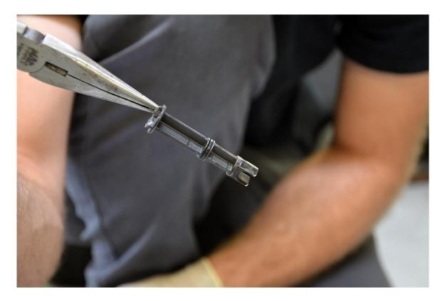
**Step 7** – Locate the factory plastic intake manifold flap linkages. Carefully remove the black plastic pins securing the linkages to the flap actuators.
