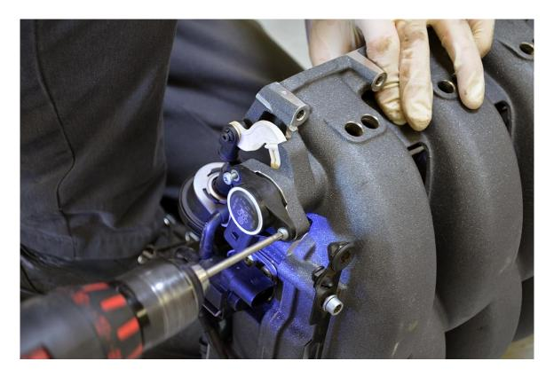
**Step 10** – The intake manifold flap rods can now be **CAREFULLY** pushed/pulled out towards the front of the car, away from the throttle body. You may need to remove the small plugs opposite the flap position sensors for easier removal.
