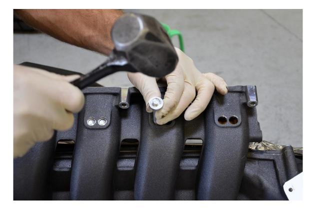
**Step 3** – Locate the T20 Torx screws that are now accessible through each of the holes for the plugs you removed. These secure the intake manifold flaps to the rod, and need to be removed for installation of the billet linkages. Remove them using a T20 Torx driver. There will be 2 for each flap, or 16 in total. **Do not lose any of them!**
