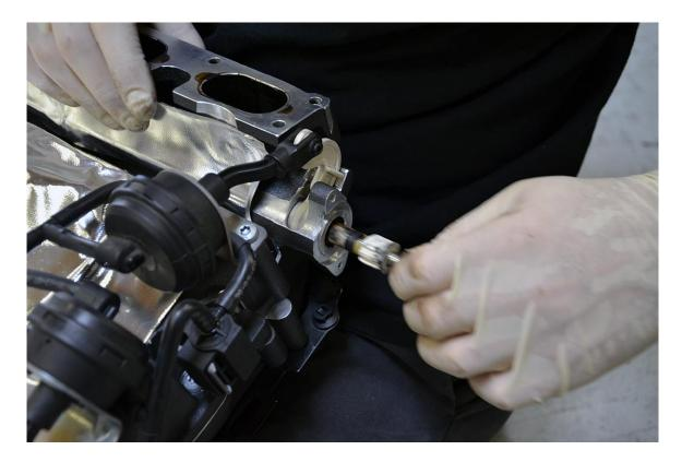
**Step 11** – With the factory intake manifold flap linkages removed, you can begin the installation of your 034Motorsport Billet Aluminum Intake Manifold Flap Linkage Pair.
