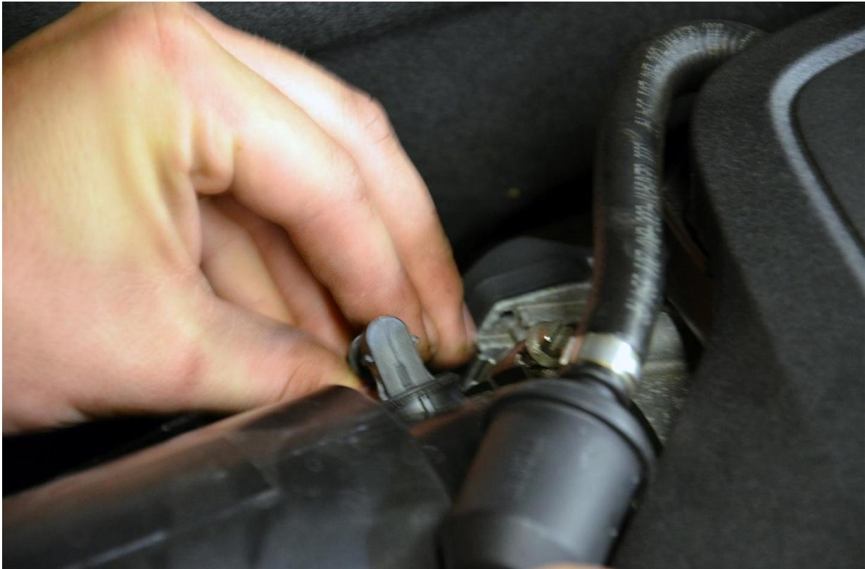
**Step 6** – Remove the stock throttle body inlet tube from the throttle body and airbox, and set aside.
