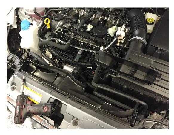
**Step 4** – The engine bay should now have plenty of room to allow for access to the stock hoses.
