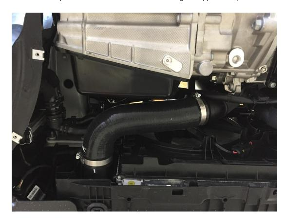
**Step 14** – Locate the intercooler outlet hose on the passenger side of the car. Remove it after loosening the factory clamps with a hose clam driver. Install the 034Motorsport Silicone Intercooler Outlet Hose using the supplied clamps.
