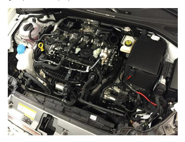
**Step 5** – Loosen the charge pipe by unscrewing the T30 screw attaching it to the right side of the intake manifold.
