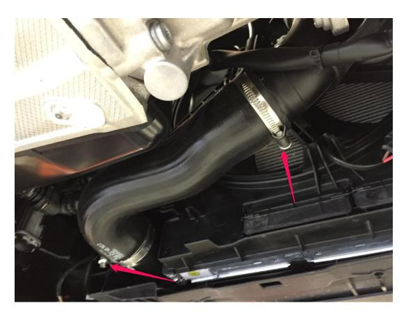
**Step 13** – Install the 034Motorsport Silicone Intercooler Outlet Hose using the supplied clamps.
