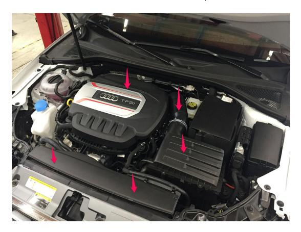
**Step 2** – To remove the air inlet duct, unclip hoses and unscrew the T2 Torx screws shown below.
