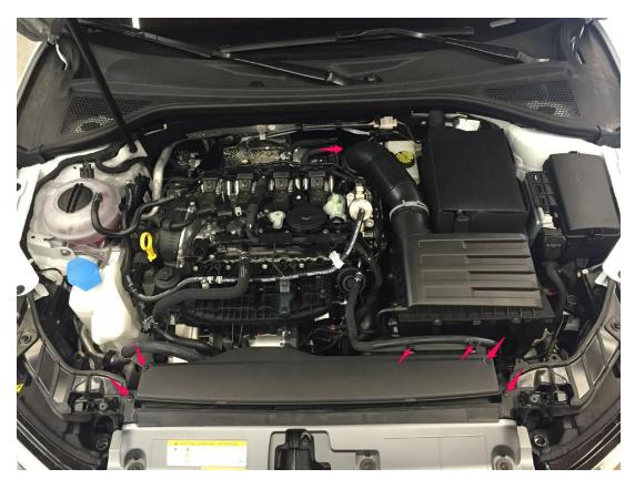
**Step 3** – You will also need to unclip the second half of the air scoop at the airbox after removing the lid, then slide out the whole piece to make room.
