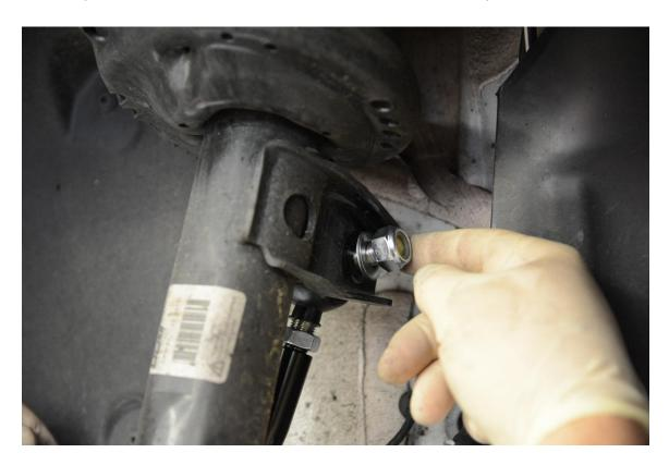
**Step 13** – Tighten nut and Allen bolt to 25 Nm using 6mm Allen Socket and 19mm Wrench.
