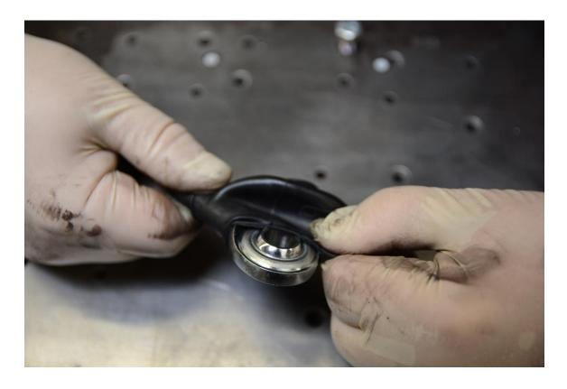
**Step 7** – (If using dust boots.) Set 034Motorsport End Link and Factory End Link side by side, and adjust the length of the 034Motorsport End Link to match. **Important:** Leave at least 8 threads exposed a the top portion (round tube, no hex) of the end link to allow for clearance at mounting tab.
