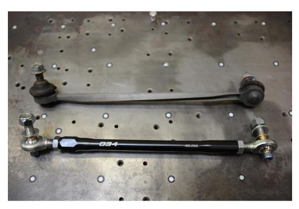
**Step 5** – (If using dust boots.) Disassemble the 034Motorsport End Links. Insert heim joint into dust boot. The boots will stretch to accommodate the heim, but avoid using sharp tools to pry at the boot.
