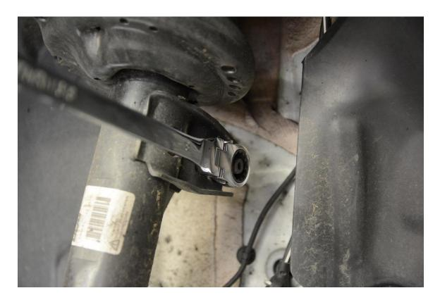
**Step 4** – (If you with to use the supplied dust boots, please proceed to Step 5.) Set 034Motorsport End Link and Factory End Link side by side, and adjust the length of the 034Motorsport End Link to match. **Important:** Leave at least 8 threads exposed a the top portion (round tube, no hex) of the end link to allow for clearance at mounting tab.
