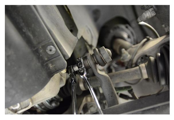
**Step 3** – Using an 18mm wrench, remove the bolt securing the top of the end link to the strut. If necessary, hold the shaft with a 6mm triple square. Remove factory end link.
