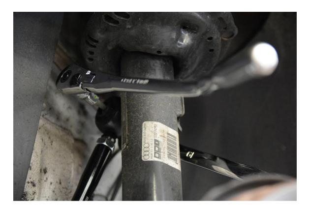
**Step 14** – Attached bottom end of link (with hex on tube) to end of sway bar. **Please Note:** You may have to pull down on sway bar to align hole with adapter. Tighten nut and Allen bolt to 25 Nm using 6mm Allen Socket and 19mm Wrench.
