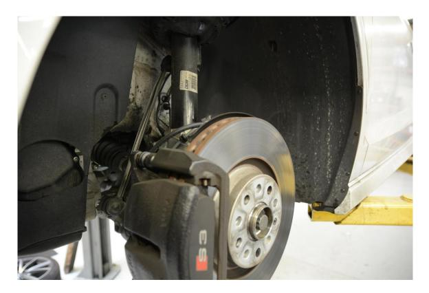
**Step 2** – Using an 18mm wrench, remove the bolt securing the bottom of the end link to the sway bar. If necessary, hold the shaft with a 6mm triple square.
