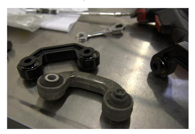
**Step 6** – Install the 034Motorsport Billet Aluminum Spherical Front Sway Bar End Links with the lower bolts in first, with the supplied washers between the bolts and end links. On B6/B7/C5 cars, the supplied M10x50 bolts thread directly into the sway bar. On the B5, the supplied M10x55 bolts go through the sway bar and are secured using the supplied M10 locknuts. **Make sure to use the correct length bolt for your vehicle to ensure proper thread engagement!**
