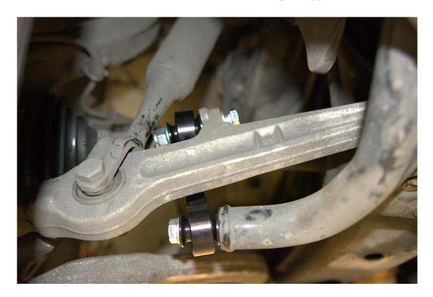
**Step 8** – Torque sway bar end link hardware to 70 Nm and marvel at your work!
