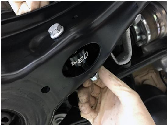
**Step 5** – With a 15mm wrench and 8mm allen, secure the top of the end link to the rear sway bar using the supplied M10 bolt, spacer, and M10 lock nut as shown below. With the suspension at full droop, this will max out the available articulation of the end links, and some force may be required to line up the holes on the sway bar and end links. With the suspension compressed at static ride height, the spherical bearings on the end links will be at their center position. Torque to 45 Nm.
