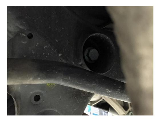
**Step 2** – Pick a side to start on - left or right: you can choose your own adventure! – and loosen the 18mm hex head bolt going through differential carrier mount, and back it out as far as possible without unthreading it completely from the nut on the other side of the mount. Let the feeling of accomplishment overcome you.
