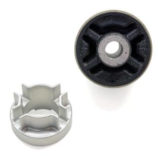
**Step 4** – Slip the shiny new 034Motorsport Differential Carrier Mount Insert over the bolt head and into the void. The 034Motorsport logo should be rotated to either the left or right side to ensure that the insert lines up with the voids.
