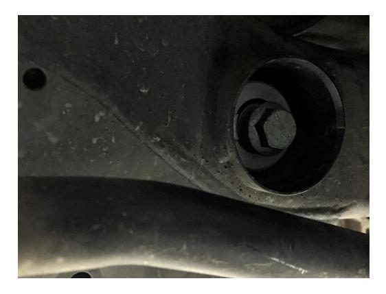
**Step 5** – Slip the provided Securing Washer between the bolt head and Rear Differential Carrier Mount Insert, locking it into the notch on the insert. Secure the 034Motorsport Differential Carrier Mount Insert & Securing Washer using the 18mm hex head bolt you loosened in <a href="Step 2">Step 2</a> and torque to 55 Nm. Yes, we provided an anchor link back to <a href="Step 2">Step 2</a> so that you wouldn't get lost. We're nice people like that over here.
