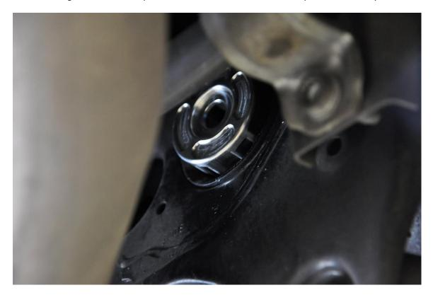
**Step 8** – Secure the 034Motorsport Differential Carrier Mount Insert using the 18mm hex head bolt you loosened in <a href="Step 3">Step 3</a>. Yes, we provided an anchor link back to <a href="Step 3">Step 3</a> so that you wouldn't get lost. We're nice people like that over here.
