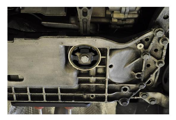
**Step 2** – Using a 21mm socket, remove the factory bolt completely in order to install the 034Motorsport Dogbone Mount Insert.
