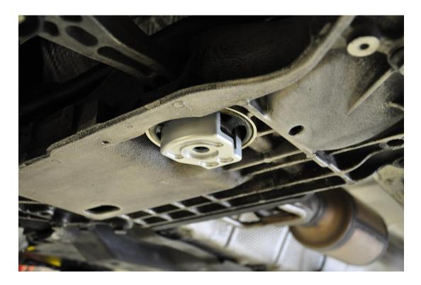
**Step 4** – Reinstall the factory dogbone mount bolt. Torque to 100 Nm.
