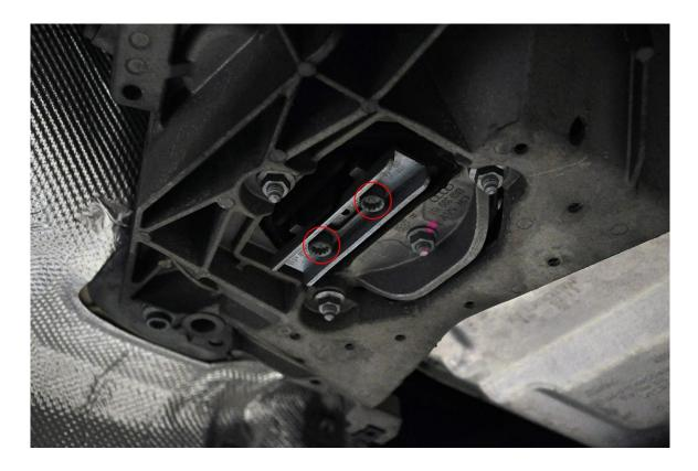
**Step 2** – Remove the two 10mm triple square bolts from the transmission mount, and remove the small bracket at the bottom. Let the feeling of accomplishment overcome you.
