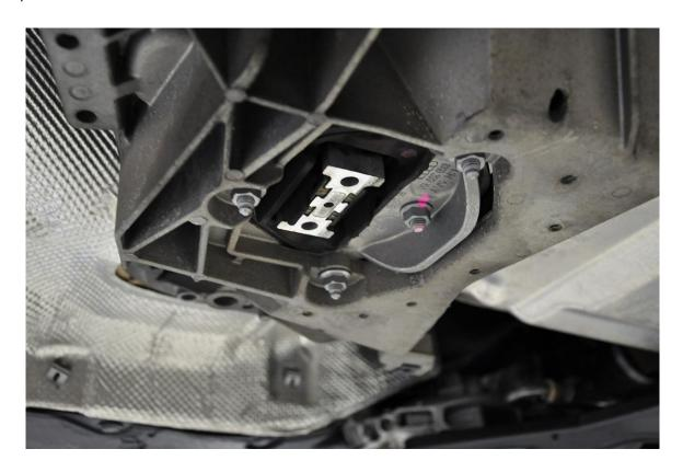
**Step 4** – Press the shiny new 034Motorsport Transmission Mount Insert into the void. The orientation of the 034Motorsport logo is not important. Or is it? It's not, but it might matter to you.
