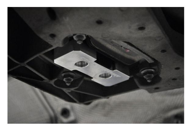
**Step 5** – Secure the 034Motorsport Transmission Mount Insert using the 10mm triple square bolts you removed in <a href="Step 2">Step 2</a> and torque to 20 Nm. Blue Loctite is recommended. Yes, we provided an anchor link back to <a href="Step 2">Step 2</a> so that you wouldn't get lost. We're nice people like that over here.
