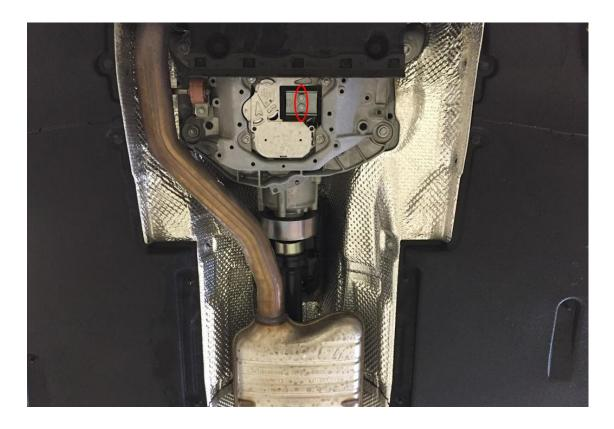
**Step 2** – Remove the two 10mm triple square bolts from the transmission mount, and remove the small bracket at the bottom. Let the feeling of accomplishment overcome you.
