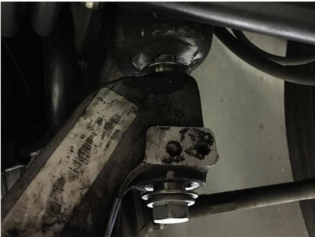
**Step 13** – In the next step, you will tighten the subframe bolts. Using a jack or support, you can raise the subframe to help align the collars before tightening, which may make the process easier.
