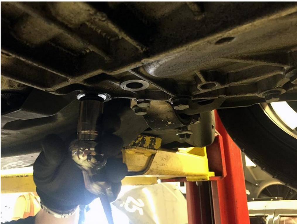
**Step 9** – With both bolts removed, attempt to slide the top collars into the top of the subframe in the correct orientation. Drop the locking collars as your hand begins to twitch. Realize you consumed far too many scoops of preworkout in Step 7. Take a deep breath. Try again, making sure that the locating features are facing up to help center the subframe on the body.
