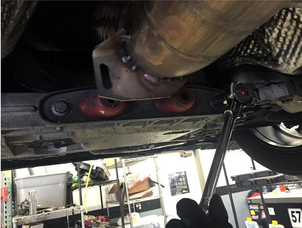
**Step 2** – Remove the two 16mm bolts securing the dogbone mount (torque arm) to the transmission. Let the feeling of accomplishment overcome you. (Not too much, though! It's nowhere near time for your post-success protein shake.)
