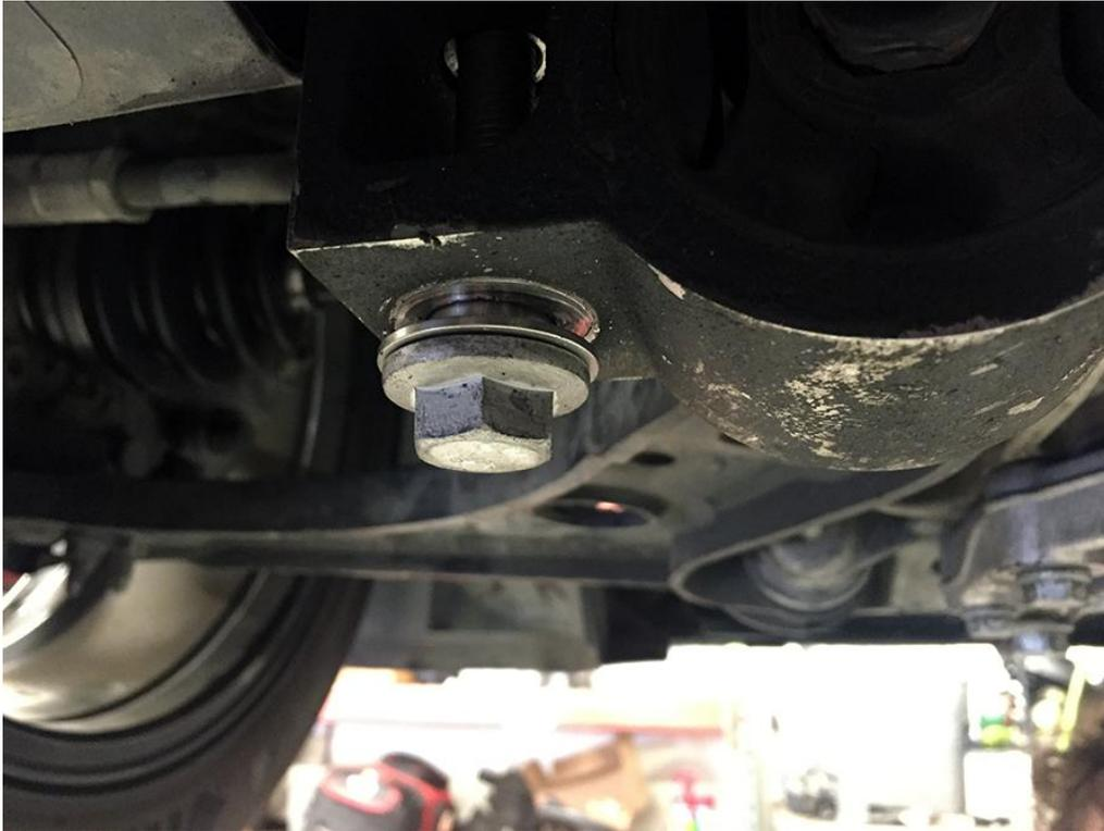
**Step 8** – Using an 18mm socket, remove both rear subframe bolts, which are probably bent. These will be replaced with the supplied constant-diameter M12x110mm subframe bolts once the locking collars are installed.
