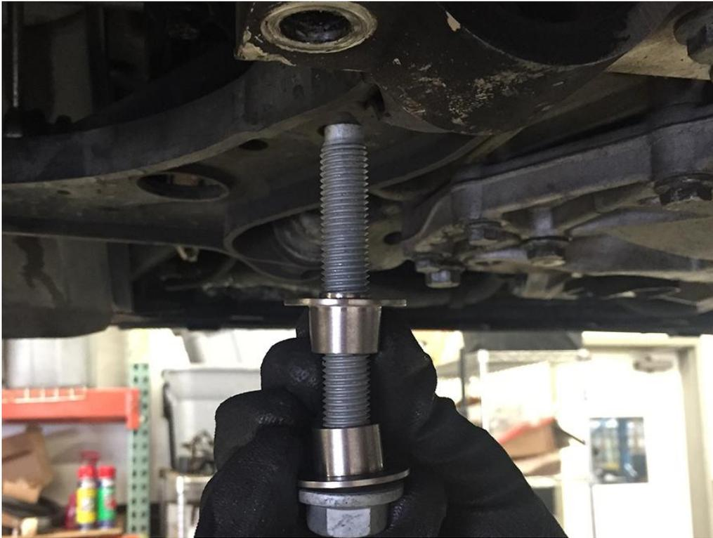
**Step 6** – Gently (jk; you're too swole to be gentle) pry the control arm bushing mount down until you have enough room to slide the top collar into place, in the top hole between the control arm bushing mount and subframe.
