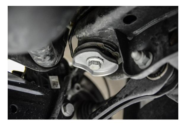
**Step 9** – Once the subframe bolt is removed, use a small pry bar to separate the factory washer from the rubber bushing.
