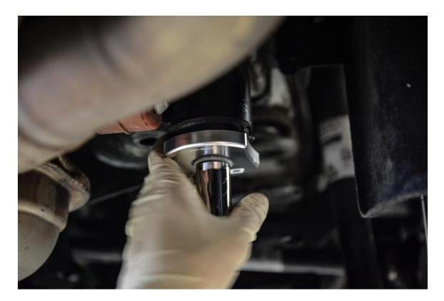
**Step 7** – Torque subframe bolt to 70 Nm + 180° Turn. (Arrows point toward the front of the car for reference)
