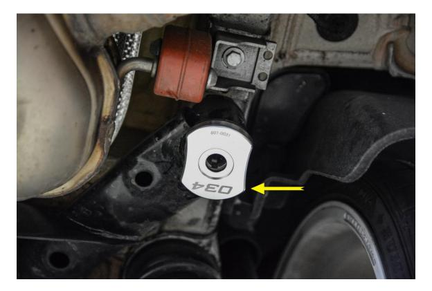
**Step 6** – Install subframe bolt using an 18mm Socket. **Note:** We recommend replacing the original subframe bolts with new pieces, as they are stretch bolts that are intended for a one-time use. **If you opt to reuse the stock bolts, torque them to 90 Nm with Blue Loctite.**
