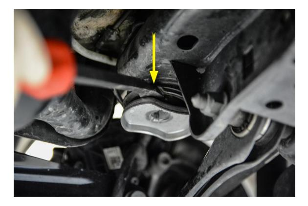
**Step 10** – Align the front-specific 034Motorsport Rear Subframe Insert (601-0030) with the voids in the factory rubber bushing.
