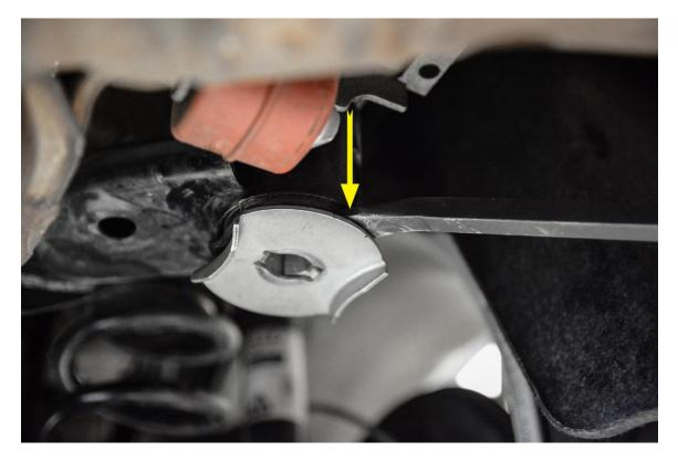
**Step 4** –Align the rear-specific 034Motorsport Rear Subframe Insert (601-0031) with the voids in the factory subframe bushing.
