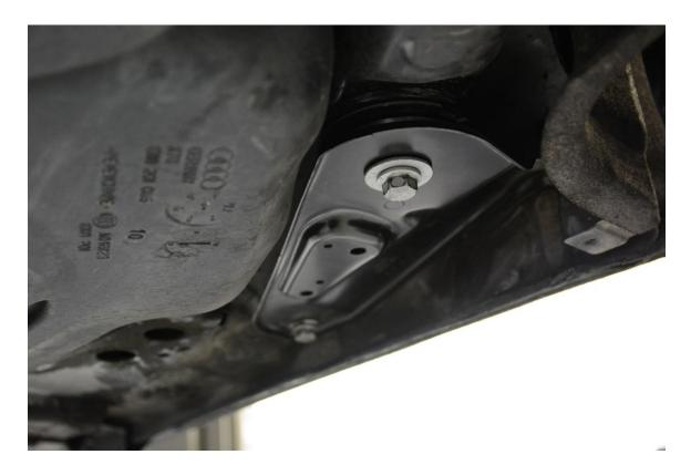
**Step 15** – Using a 16mm Socket, remove the two bolts securing the subframe mount bracket to the chassis.
