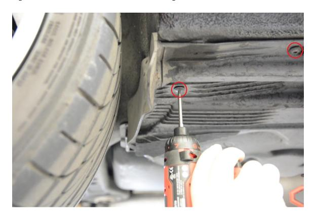
**Step 13** –Unclip the front portion of the plastic cover as shown below.
