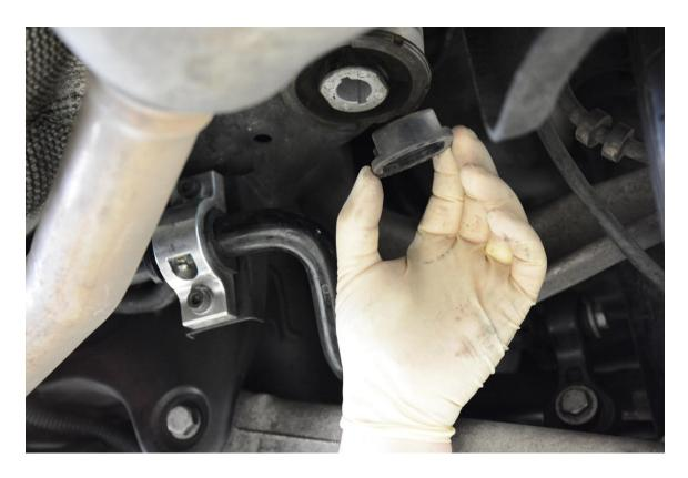
**Step 5** –Apply silicone grease to the insert as pictured below.
