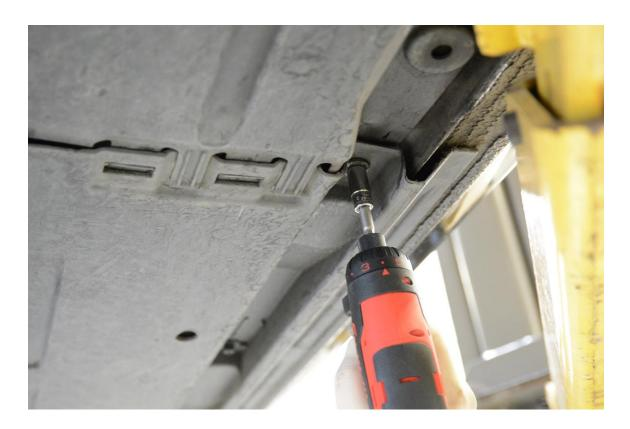
**Step 12** –Using a T20 Torx driver, remove the two bolts securing the rear subframe cover.
