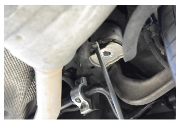
**Step 3** –Remove the factory washer and set aside.
