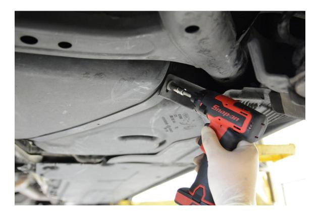
**Step 10** – Using a 10mm Socket, loosen the inner front nut securing the rear subframe cover.
