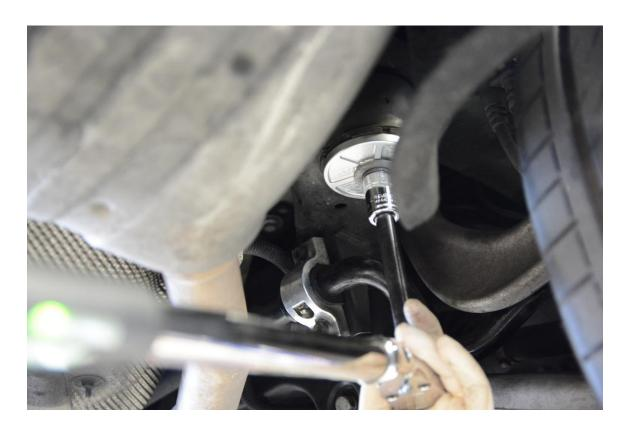
**Step 9** - Using a 10mm Socket, remove the rear-most nut securing the rear subframe cover.
