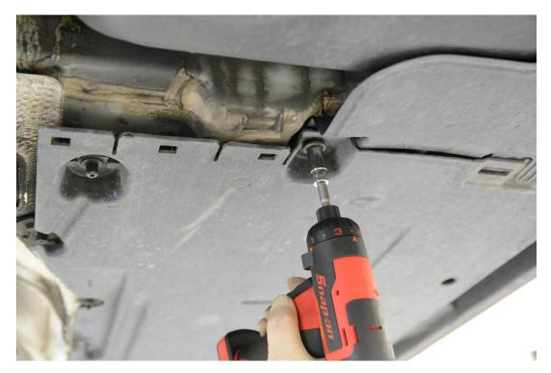
**Step 11** – Using a 10mm Socket, loosen the outer front nut securing the rear subframe cover.
