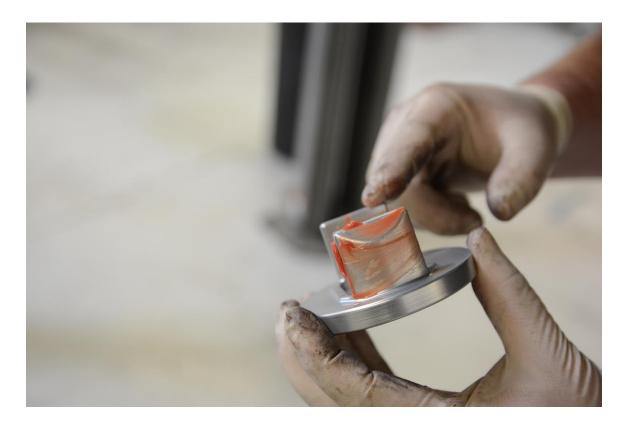
**Step 20** – Align the 034Motorsport Front Subframe Insert (601-0033) with the voids in the factory subframe bushing.
