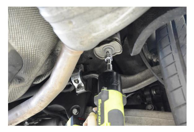
**Step 2** – Once the subframe bolt is removed, use a small pry bar to separate the factory washer from the rubber bushing.
