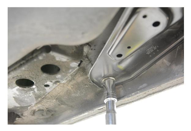
**Step 16** – Using an 18mm Socket, remove the bolt securing the front of the rear subframe to the chassis, and remove the steel subframe mount bracket.
