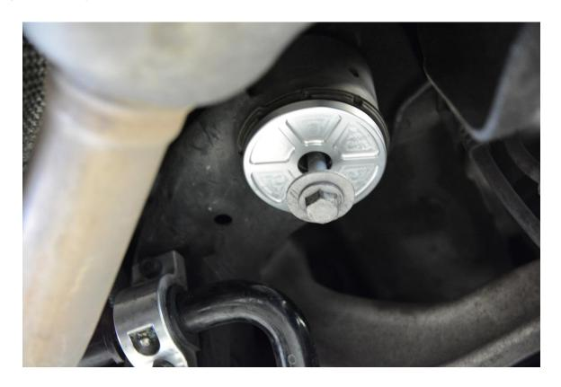
**Step 8** – Torque new subframe bolt to 115 Nm + 90° Turn. **If you opt to reuse the stock bolts, torque them to 120 Nm with Blue Loctite.**
