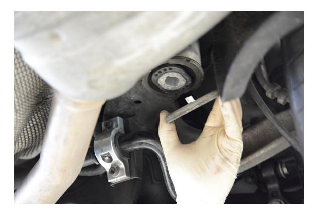
**Step 4** –Remove the factory plastic isolator and set aside.
