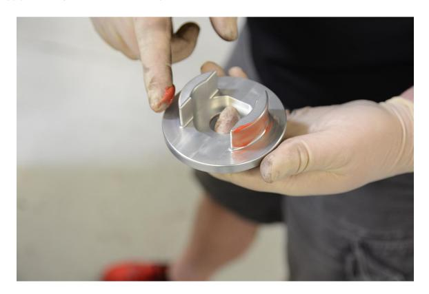
**Step 6** – Align the 034Motorsport Rear Subframe Insert (601-0034) with the voids in the factory subframe bushing.
