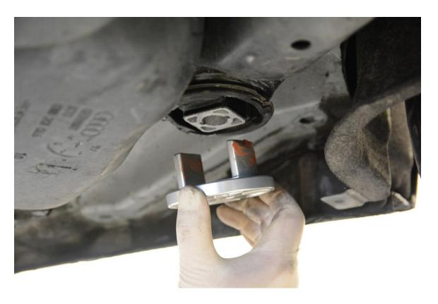
**Step 21** – Reinstall the subframe mount bracket and bolt, tightening loosely to allow for alignment of the two additional bolts.
