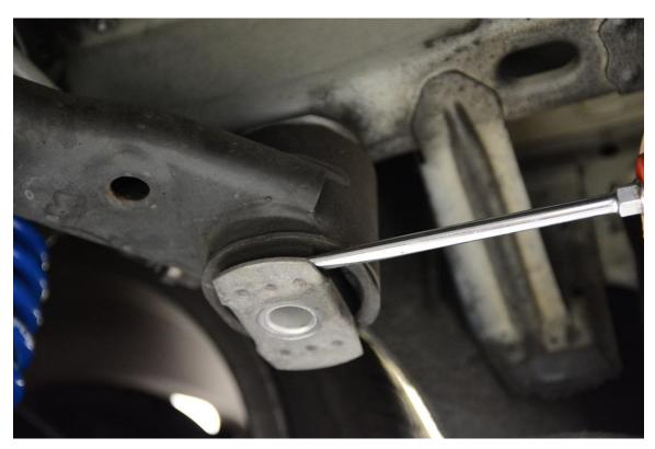
**Step 4** –Remove the factory washer and set aside.
