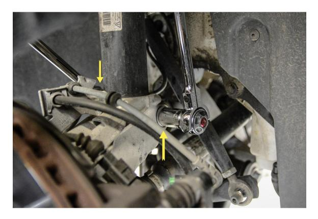
**Step 20 - Using 13mm socket, t**orque upper 3 strut bolts to <u>15 Nm + 90° turn</u>.
