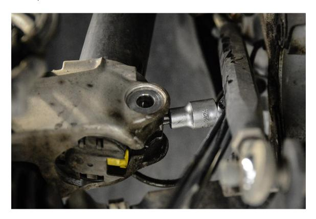
**Step 10C** – Once lower strut bolt and nut are removed, use a Spreader Socket to separate the strut housing from the lower knuckle. Spreader Socket shown inserted into lower knuckle below.
