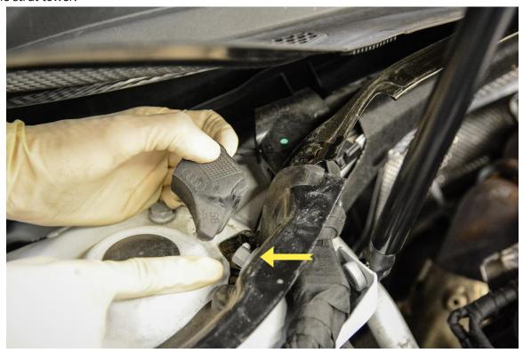
**Step 4** – Using a 10mm Socket, remove the bolt securing the cowl dust shield to the strut tower
