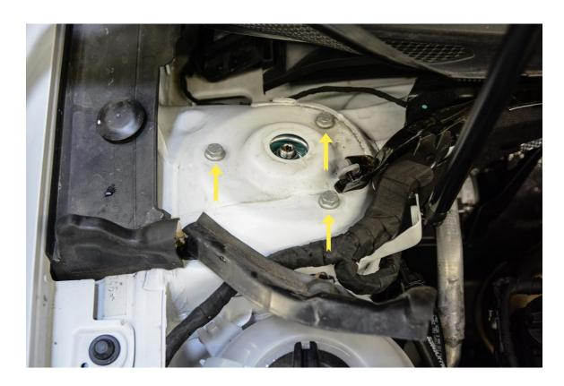
**Step 12 -** Now the complete strut assembly should be free from the car. Use spring compressors to remove any spring tension from the upper spring hat. Once spring pressure is eliminated from the upper spring perch, you can safely remove the strut mount. Use a 21mm (or 13/16" Standard) Spark Plug Socket and 7mm Allen to remove the upper strut nut.
