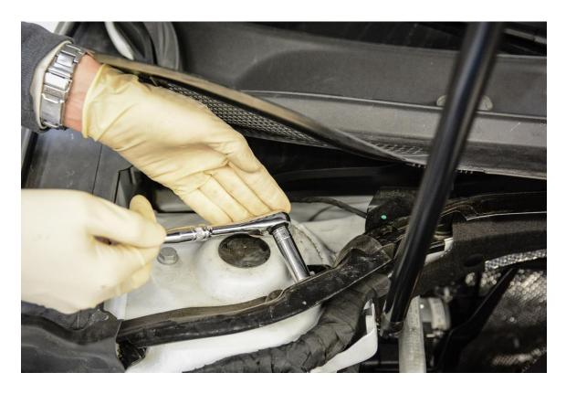
**Step 5** – With the dust shield out of the way, you'll notice the easy access to the 3 strut mount bolts for later.
