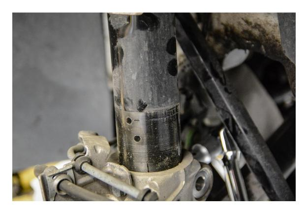
**Step 19 -** Once strut assembly is bottomed out in the knuckle, reinstall bolt and nut using 14mm Triple Square and 18mm Socket respectively. Torque to <u>70 Nm + 90° turn</u>.
