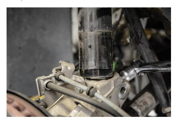
**Step 11 -** Once the lower portion of the strut assembly is free from the knuckle, use a 13mm Socket to remove the 3 strut mount bolts.
