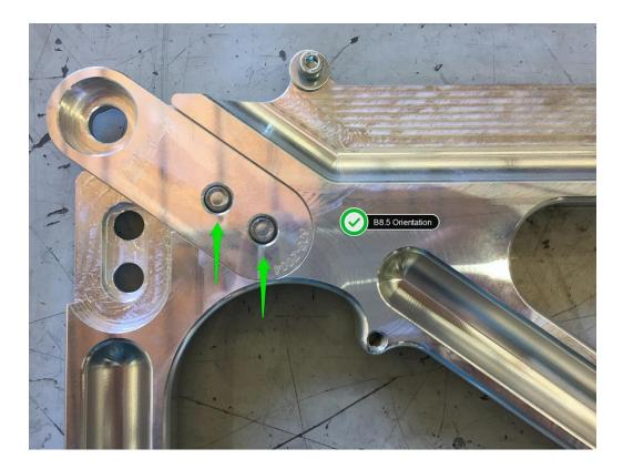
**Step 7** – Install the 034Motorsport X-Brace using new bolts. **(Facelift)** Torque the six M12 hex head bolts to 90 Nm + 135 Degrees. **(Pre-Facelift)** Torque the four M12 hex head bolts to 90 Nm + 135 Degrees. Torque the two M12 triple-square bolts to 90 Nm + 90 Degrees. Marvel at your work!
