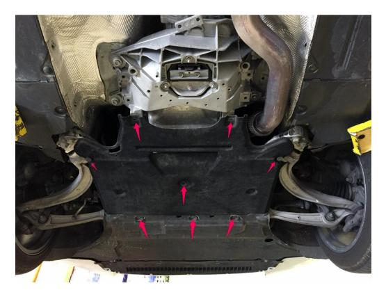
**Step 2 – (Facelift)** Remove the two plastic factory clips securing the power steering cooler lines to the stock subframe brace. (**Pre-Facelift**) Use a 10mm socket to remove the nut securing the power steering cooler to the subframe brace.
