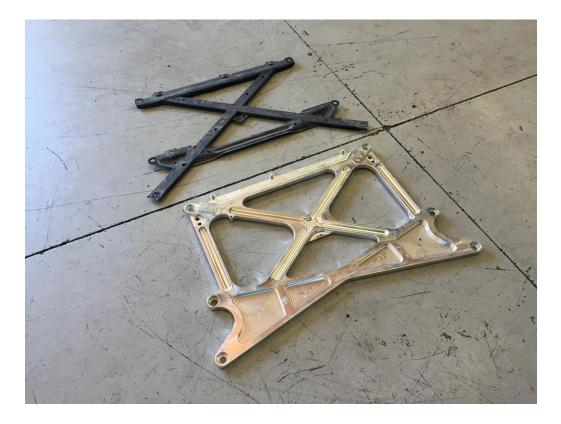
**Step 6** – In this step, install the Modular X-Brace Inserts in the proper orientation for your vehicle. Torque the provided M10 screws to 55 Nm using a 6mm allen driver. **(Facelift)** The inserts should install diagonally, as pictured below. **(Pre-Facelift)** The inserts should be installed straight up and down.
