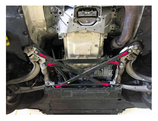
**Step 4** – Remove the factory subframe brace, and set aside. **(Pre-Facelift)** You must remove the threaded power steering cooler hose mounting bushing from the factory subframe brace using a 19mm box wrench, and transfer it over to the matching hole on the 034Motorsport X-Brace.
