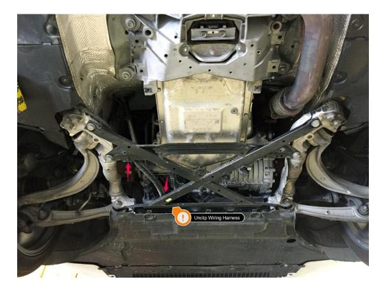
**Step 3** – Support the subframe brace with one hand to ensure that it doesn't fall on your head. Using the 18mm socket, 14mm triple square, and your superhuman strength, loosen the bolts that attach the stock subframe brace.
