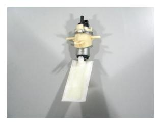
4 – wire in the supplied electrical connector (red-to-red and black-to-brown) and push the PTFE hose onto the assembly inlet. Secure the pump in place using the OE rubber isolators
