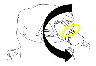
Ensure the cavity is free from debris using avoiding shifting dirt into the passages.
