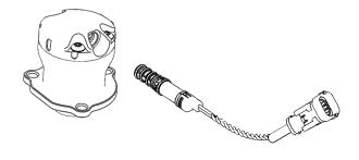
Tighten the new solenoid into the EM series BOV ensuring the wrench is on the metallic portion of the solenoid.
