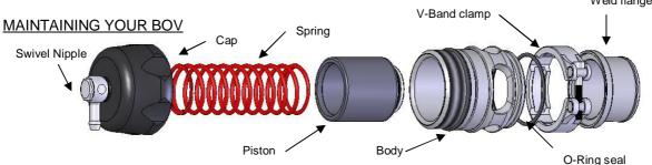
Turbosmart recommends that the following maintenance procedure is carried out at six monthly intervals. Regular maintenance will ensure that your BOV is operating at its peak and will extend the working life of the product.
