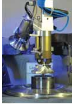
Forged-milled compressor wheel production
